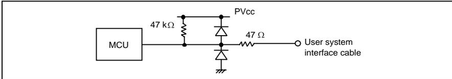
**Figure 7.1** Default User System Interface Circuit
