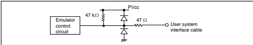
**Figure 7.2** User System Interface Circuit for Mode Pins
