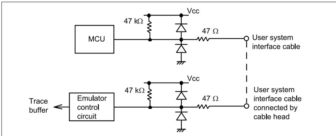
**Figure 2.5** IRQ0–IRQ7 and WAIT User System Interface Circuit
