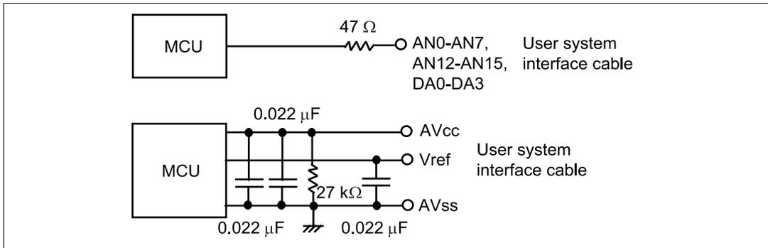
**Figure 2.4** User System Interface Circuit for AN0 to AN7, AN12 to AN15, DA0 to DA3, AVcc, AVss, and Vref Signals
