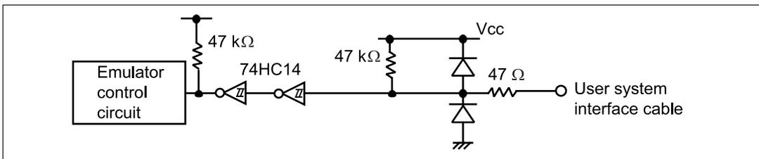
**Figure 2.3** User System Interface Circuit for RESET
