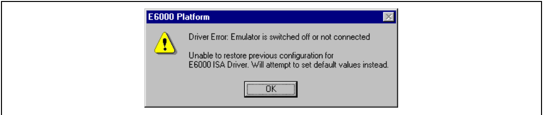
Figure 2.4 Faulty Connection Message
