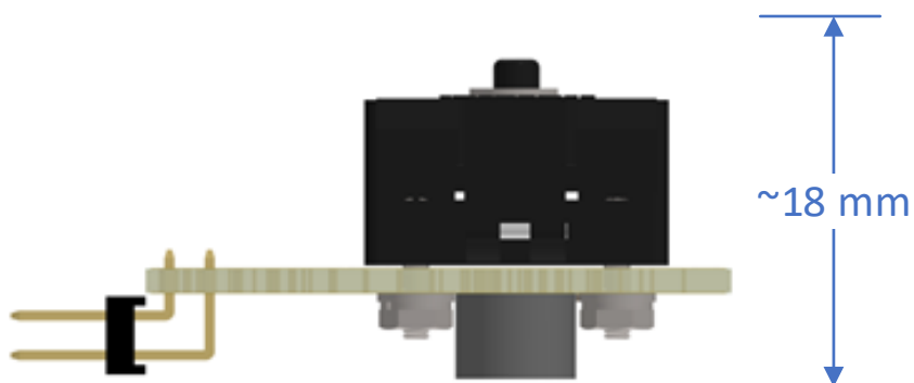
Figure 5. Board Assembly Side View Dimensions
