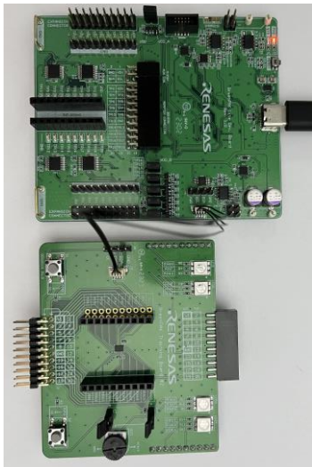
Figure 20. Training Board #2 Connection
