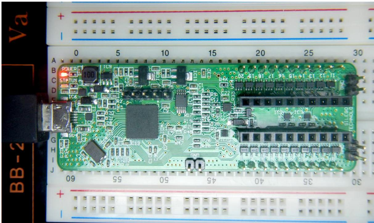
**Figure 3: Breadboard with GreenPAK DIP Development Board**
