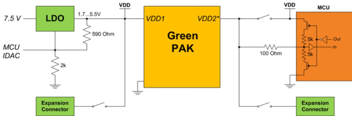
Figure 6: Schematic Connection of the V<sub>DD</sub> Pin
