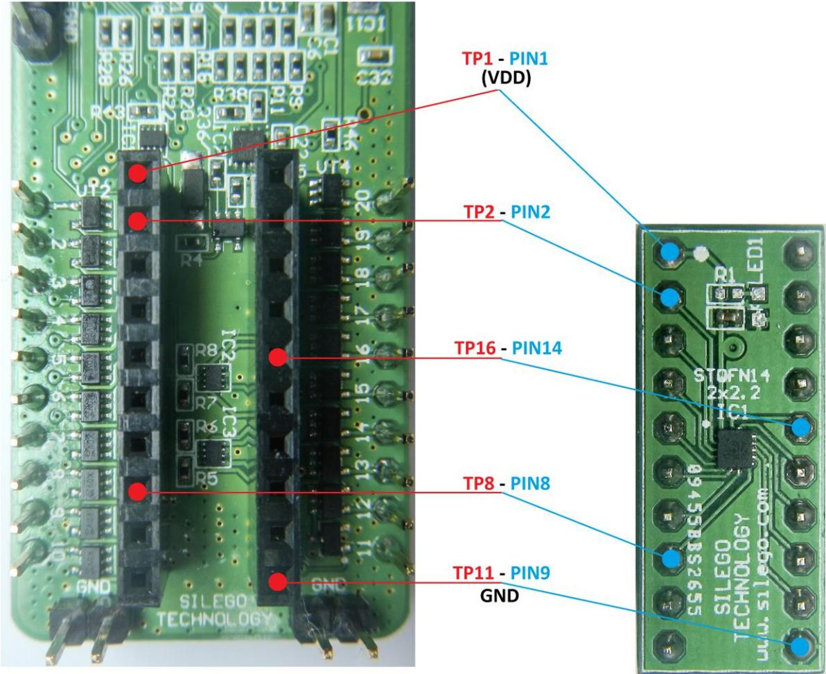
Figure 9: Pins and TPs Accordance (for SLG46534)
