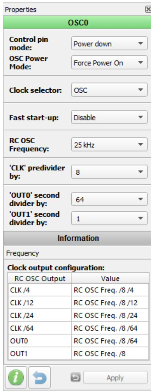
Figure 16: Oscillator Properties
