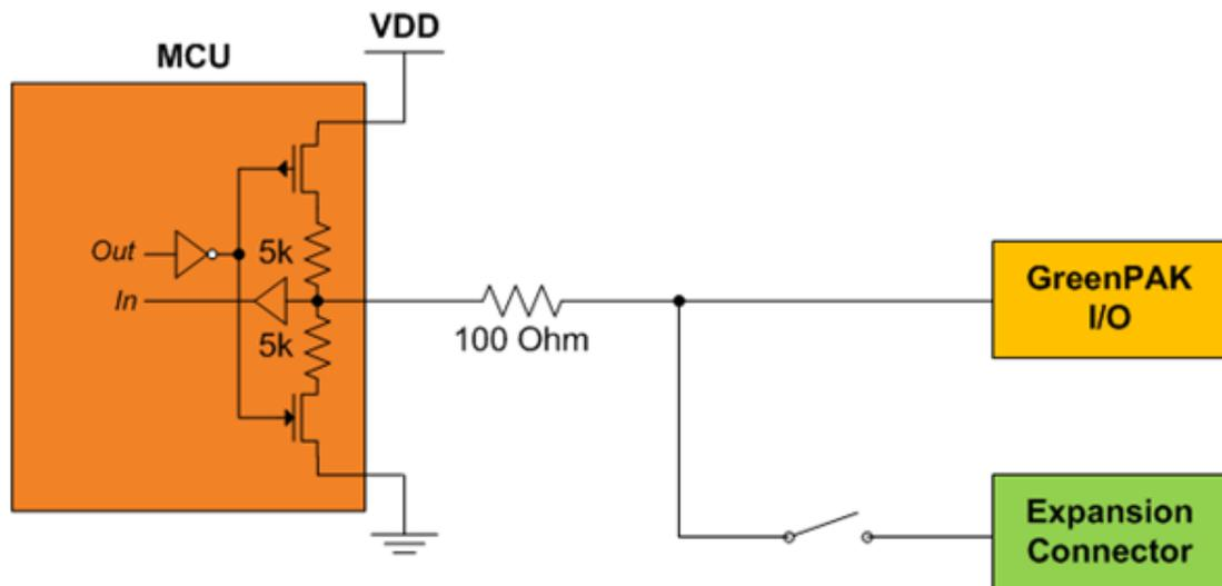
Figure 7: Schematic Connection of the Data Pin
