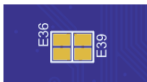
Figure 22. Jumper for main clock oscillation circuit (Bottom view)
