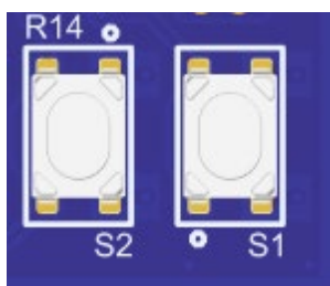
Figure 19. User Switch (S1) and Reset Switch (S2) (Top view)
