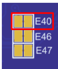
Figure 20. Jumper for User Switch (S1) (Bottom view)
