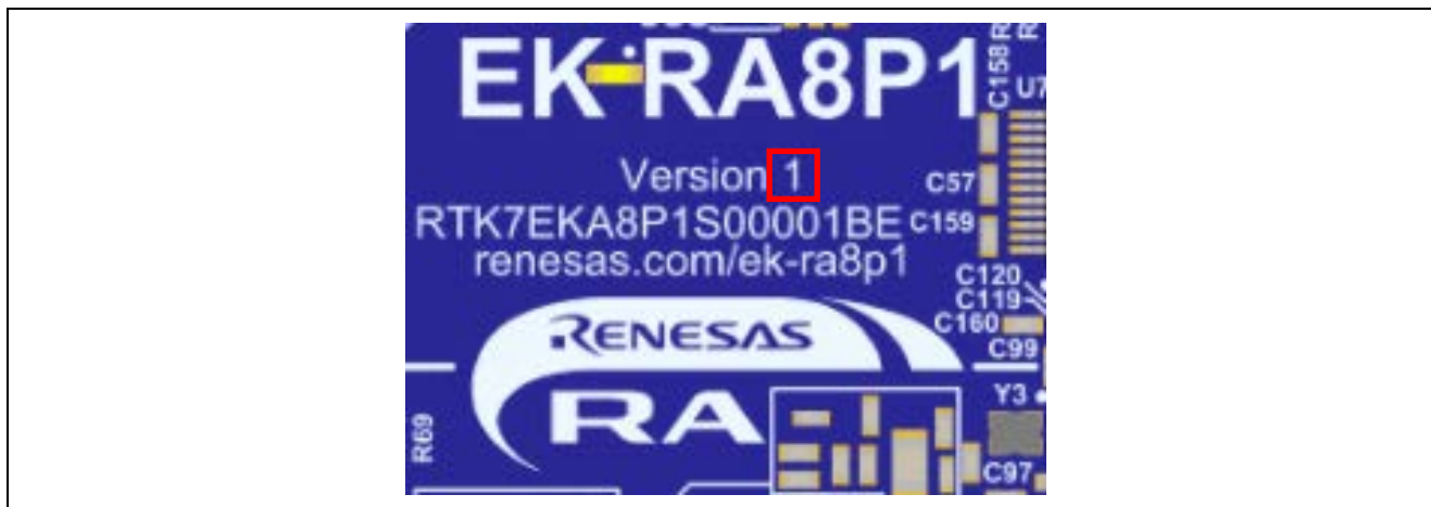
Figure 2. Identification of the Kit Version Number on the EK-RA8P1 Board
