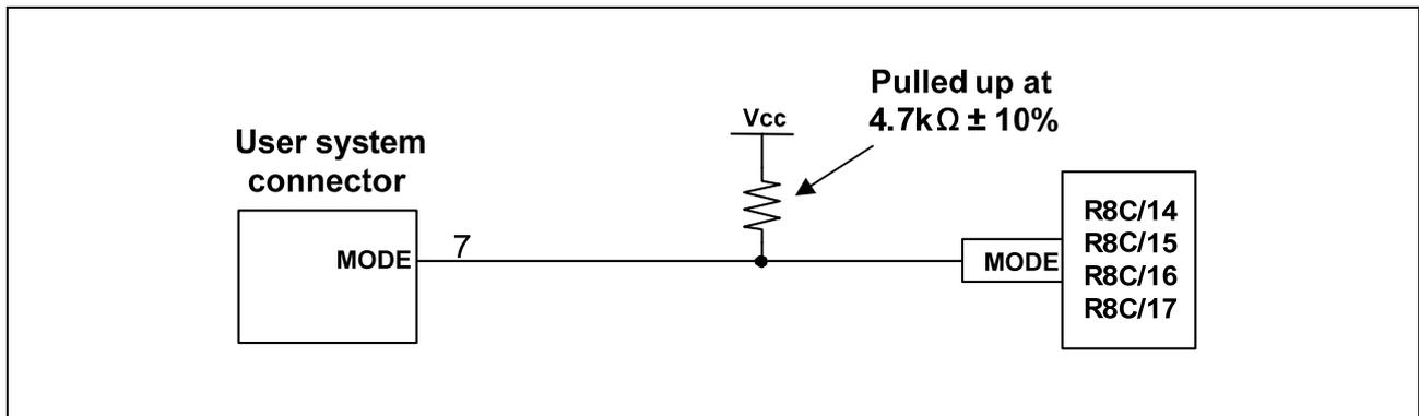
Figure 5.2 E8 Emulator and MODE Pin Connection
