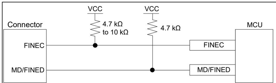
**Figure 2.25 Connection of the FINEC and MD/FINED Pins**
