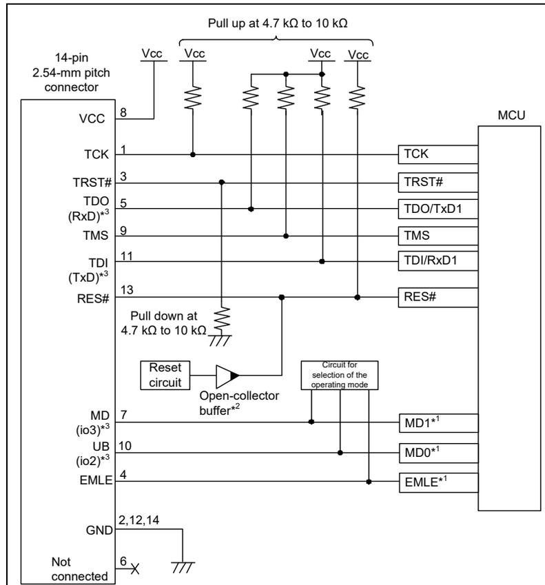
**Figure 2.11 Example of Connection between the 14-Pin Connector and MCUs of the RX63x, RX64x, RX65x, RX66x, RX67x, RX71x, RX72x and RX26T Groups in JTAG Interface Connection (for Debugging and Flash Programming)**
