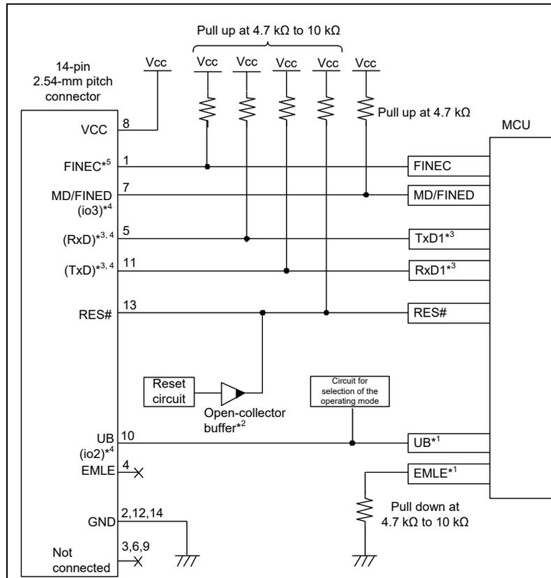
**Figure 2.12 Example of Connection between the 14-Pin Connector and MCUs of the RX63x, RX64x, RX65x, RX66x, RX67x, RX71x, RX72x and RX26T Groups in FINE Interface Connection (for Debugging and Flash Programming)**
