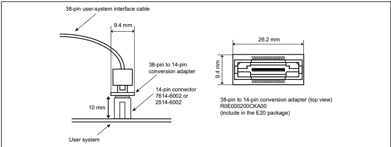
**Figure 2.2 Connecting the User System Interface Cable to the 14-Pin Connector of the E20 Emulator**
