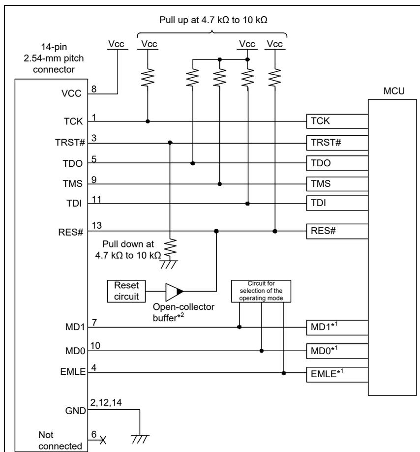
**Figure 2.7 Example of Connection between the 14-Pin Connector and MCUs of the RX610 Group in JTAG Interface Connection (for Debugging)**
