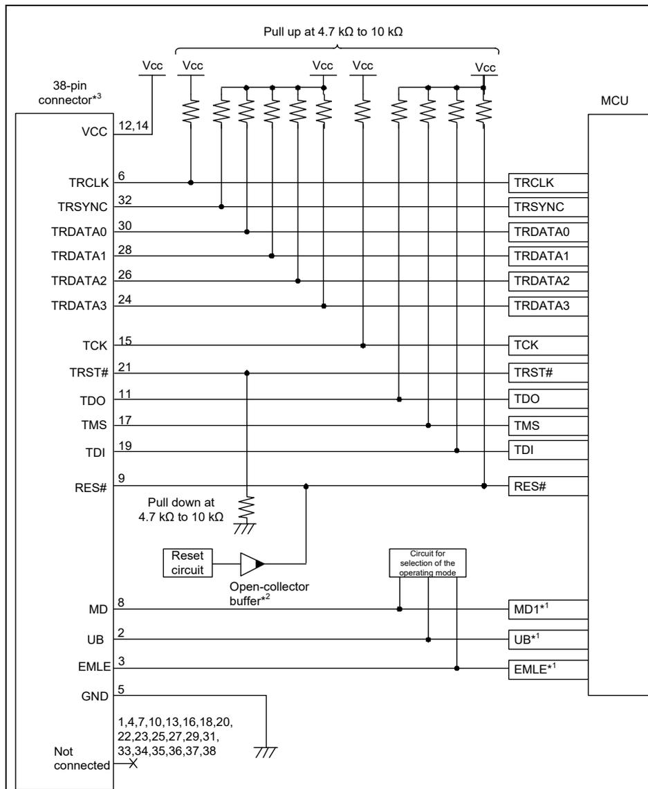
**Figure 2.16 Example of Connection between the 38-Pin Connector and MCUs of the RX63x, RX64x, RX65x, RX66x, RX67x, RX71x, RX72x and RX26T Groups in JTAG Interface Connection (for Debugging and Flash Programming)**
