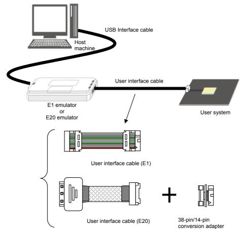
**Remark** To use it with the E20, connect the 38-pin/14-pin conversion adapter to the user interface cable (E20). 38-pin is not supported.
