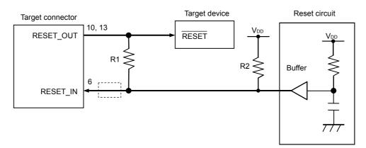
Remark Make the resistance of R1 at least ten times that of R2, R1 being 10 k $\Omega$  or more. Pull-up resistor R2 is not required if the buffer of the reset circuit consists of CMOS output. The circuit enclosed by a dashed line is not required when only flash programming is performed.
