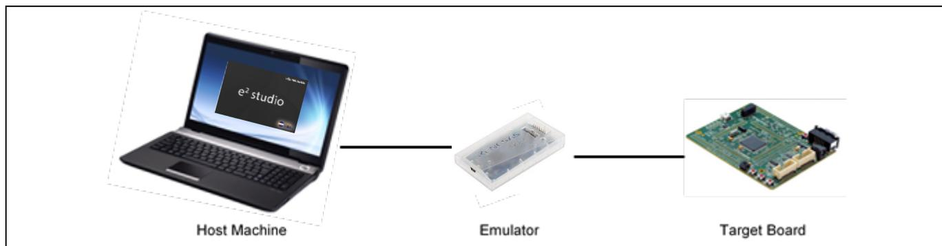
Figure 1-1 System Configuration
