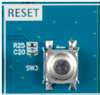
Figure 21. Reset Push-button Switch
