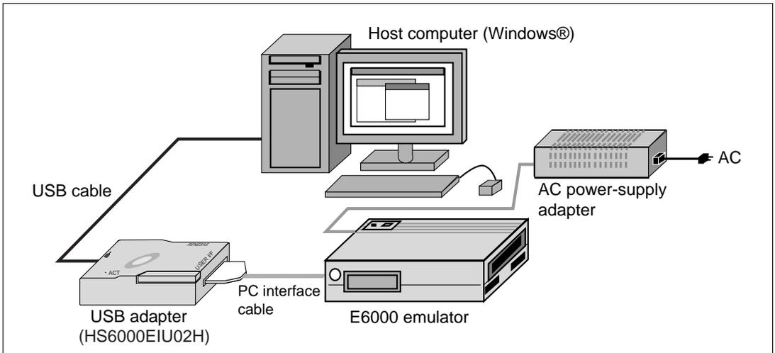
**Figure 1.1 System Configuration of E6000 Emulator Connection**
