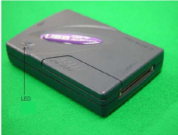
**Figure 5.1 LED for Displaying the Communication State**
