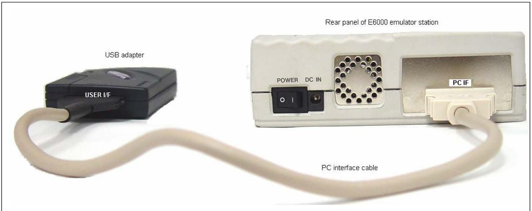
**Figure 3.2 Connecting USB Adapter to E6000 Emulator**
