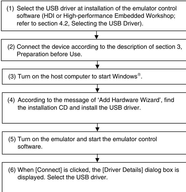
**Figure 4.1 Setup Procedures**
