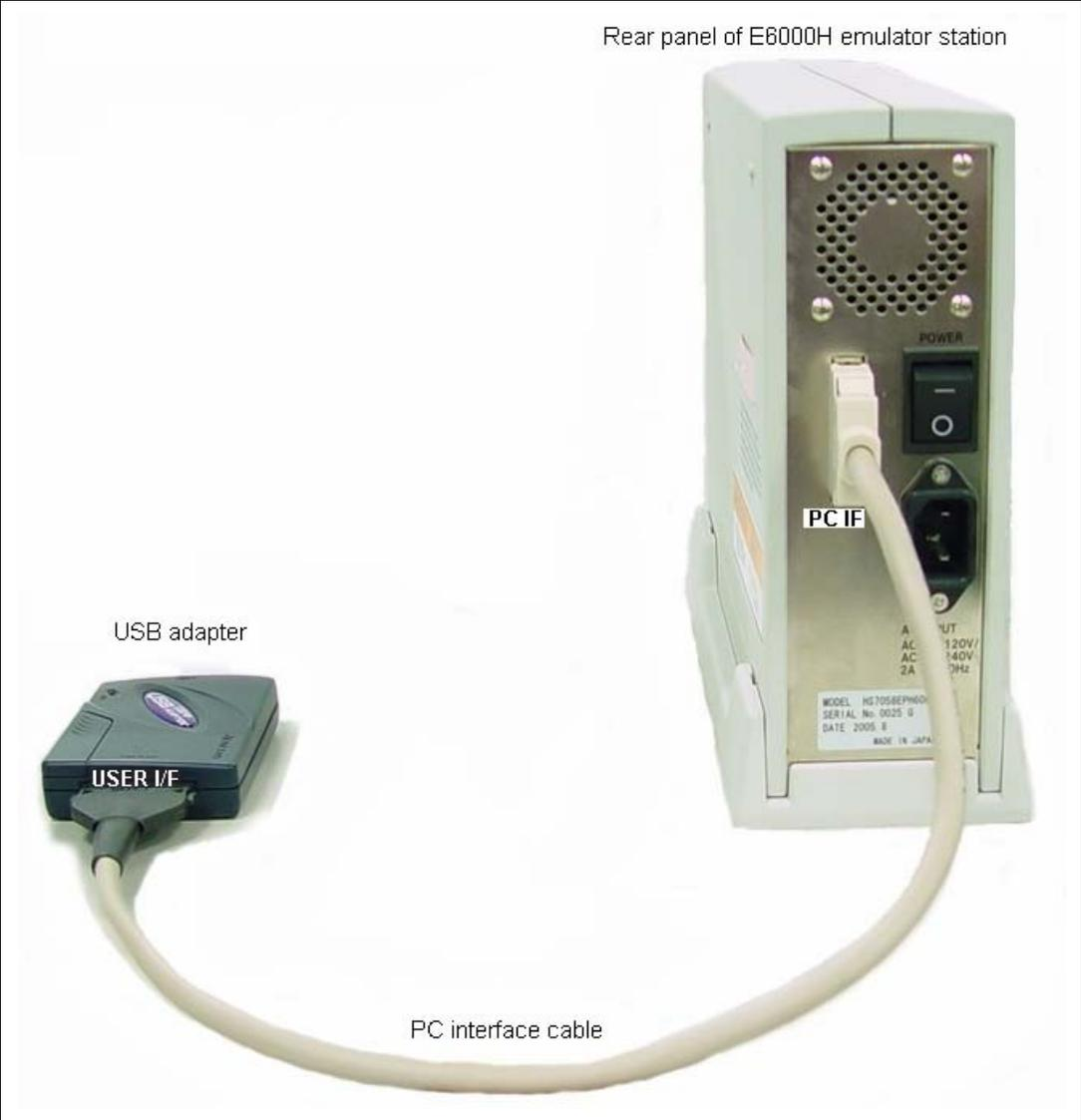
**Figure 3.3 Connecting USB Adapter to E6000H Emulator**
