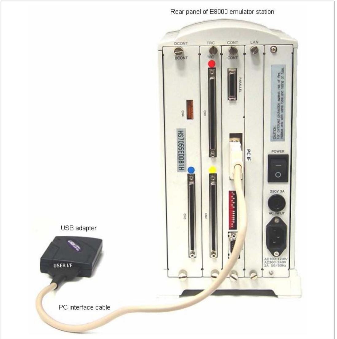
**Figure 3.4 Connecting USB Adapter to E8000 Emulator**
