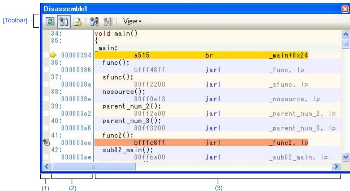
Figure A-27. Disassemble Panel (When Disassemble Display Mode Is Selected)
