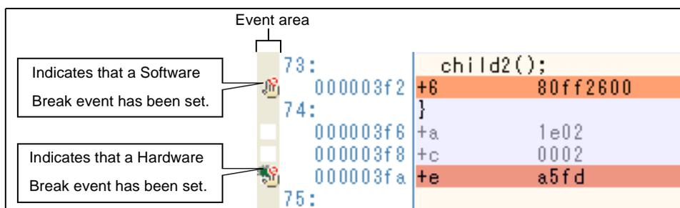
**Figure 2-78. Example of Setting Hardware Break Event (Execution Type) in Events Panel**
