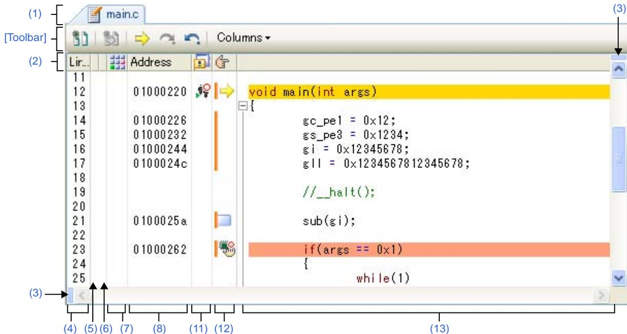
Figure A-16. Editor Panel (When Code Coverage Measurement Result Is Displayed) [Simulator]
