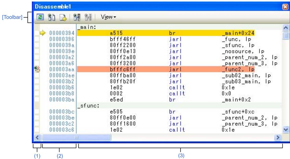
Figure A-28. Disassemble Panel (When Code Coverage Measurement Result Is Displayed) [Simulator]
