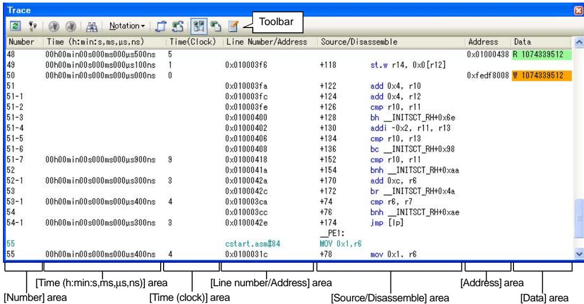
Figure 2-111. Display Trace Data (Trace Panel [Simulator])
