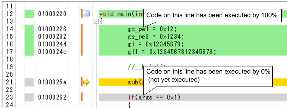
Figure 2-125. View of Code Coverage Measurement Result (Disassemble Panel)
