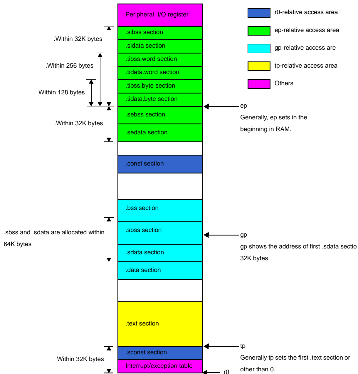
Figure 5-4. Example of Memory Allocation to Various Sections by CX (With Internal ROM)
