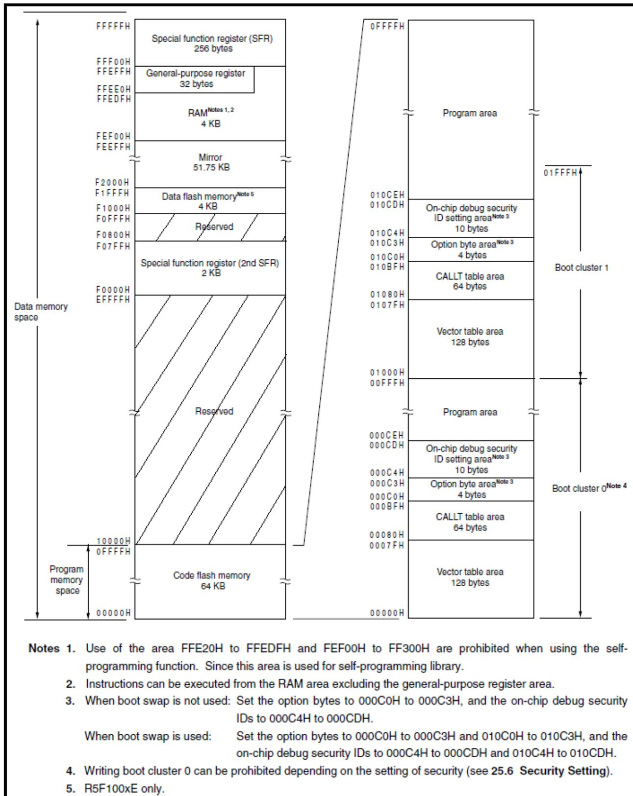
Figure 8-1: MCU Address Space Diagram
