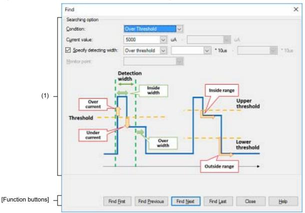
Figure A.74 Current Consumption Measurement Search Dialog Box
