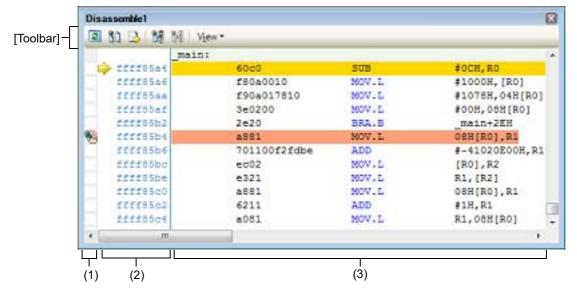
Figure A.28 Disassemble Panel (When Code Coverage Measurement Result is Displayed) [Simulator][E20 [RX71M, RX65x, and RX64M]
