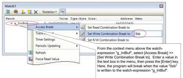
Figure 2.116 Example of Setting a Break Event (Access-related) on a Watch-expression [Simulator]
