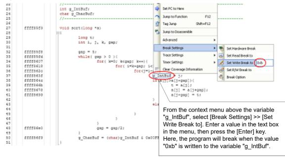
Figure 2.113 Example of Setting a Break Event (Access-related) on a Variable in the Source Text [Simulator]
