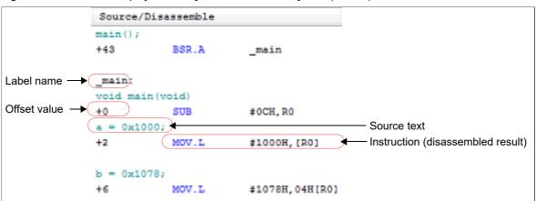
Figure A.38 Contents Displayed in the [Source/Disassemble] Area (Default)
