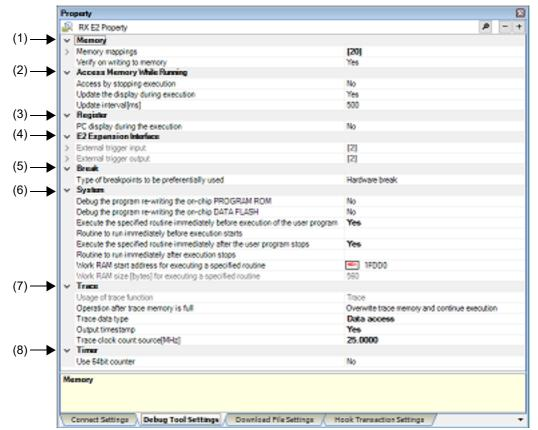
Figure A.16 Property Panel: [Debug Tool Settings] Tab [E20(Serial) [RX600 Series]]
