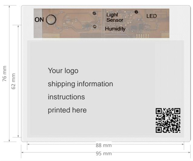
BLE Smart Asset Tracking Label dimensions ~ 95 x 76 x 2.5 mm
