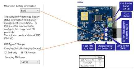
In "BMS" setting, this EVB frequently retrieves battery related information from RAJ240100 Filefish EVM. In this operating mode, this EVB uses the information obtained from RAJ240100 Filefish EVM instead of SW1B value to configure the On-Board Charger.
