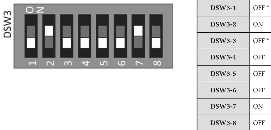
Figure 4-25: SCIF Download MODE(DSW3) on RZ/N2H
