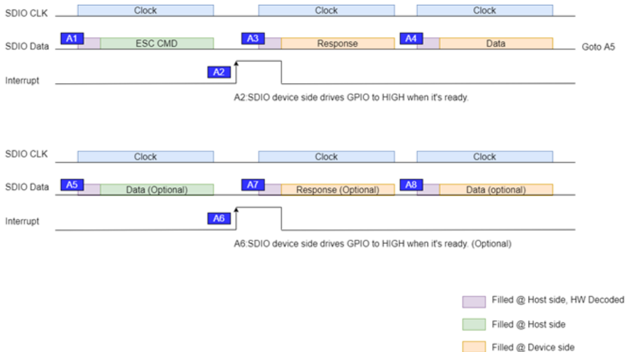
Figure 26. SDIO host to device sequence (ESC command)
