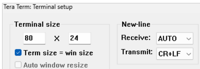
Figure 17. Tera Term New-line configuration
