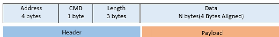
Figure 3. Basic SPI message format
