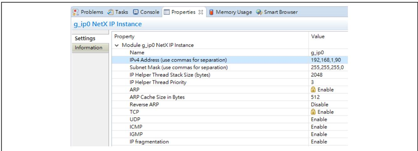
Figure 4.1 The properties view of NetX IP instance module
