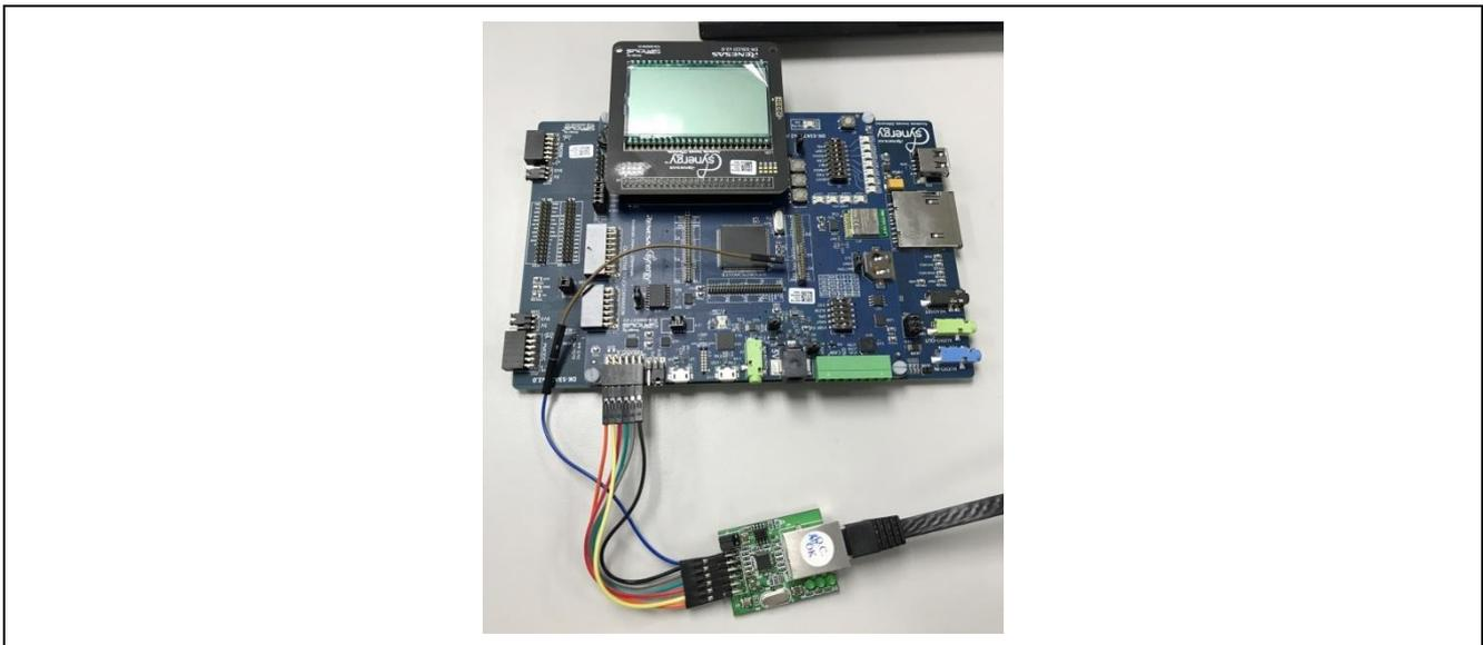
**Figure 2.1 shows the DM9051 Demo Board connected to the PMODA connector on DK-S3A7**
