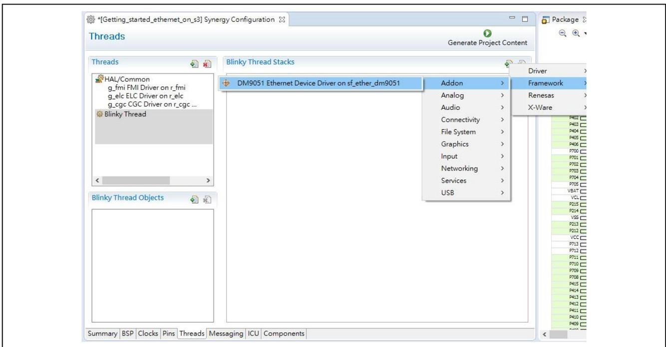
7. Add SPI Driver on r\_sci\_spi under DM9051 Ethernet Device Driver
