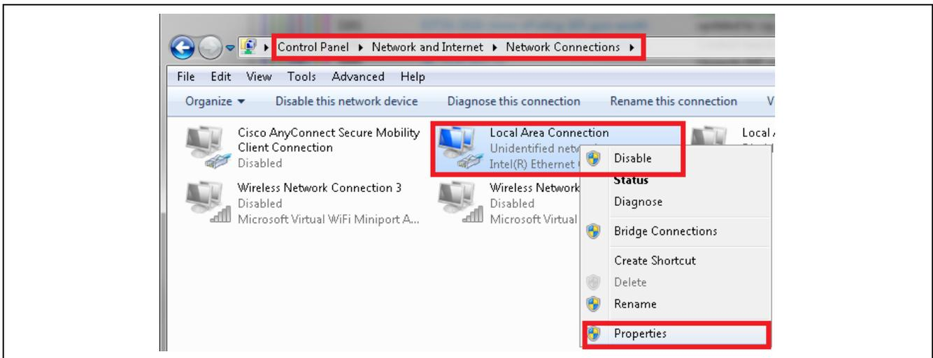
Figure 4.2 Configure the Ethernet port of your PC to static IP address in order to test the Board
