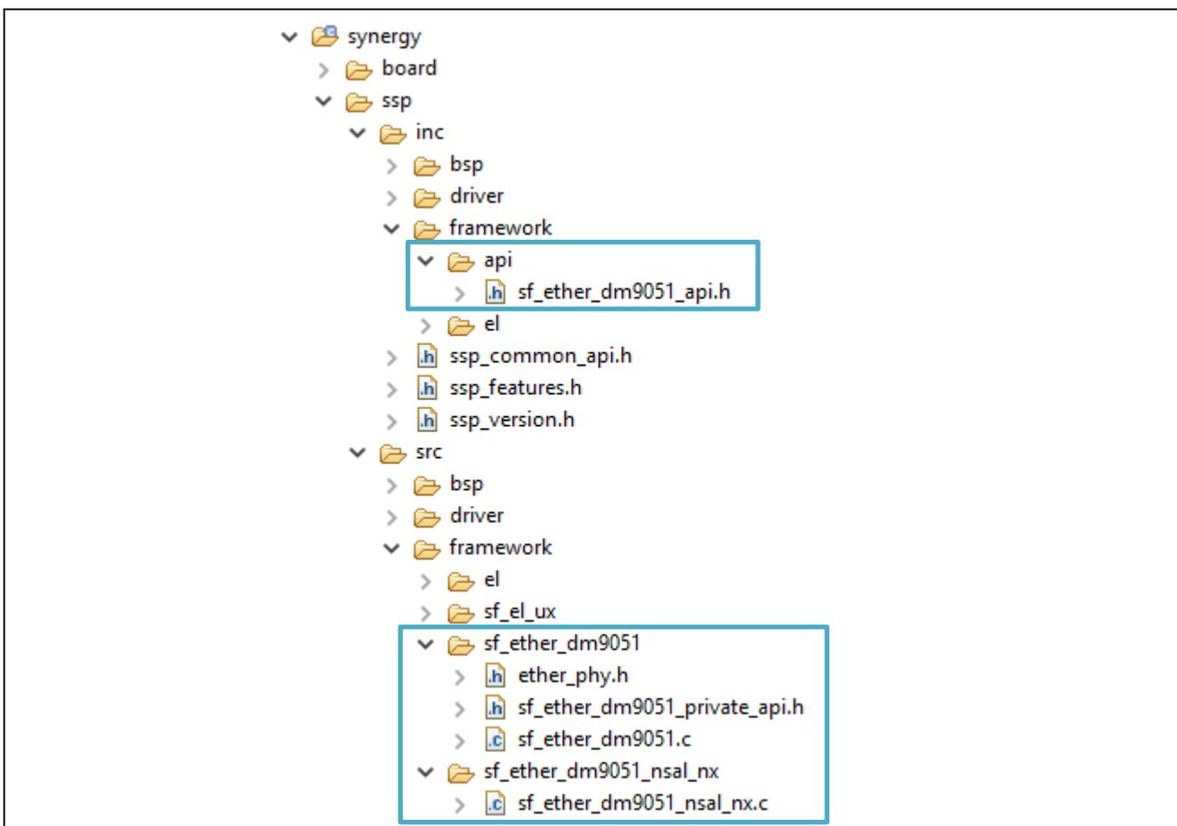
Figure 5.3 DM9051 add-on code and its driver directory structure
