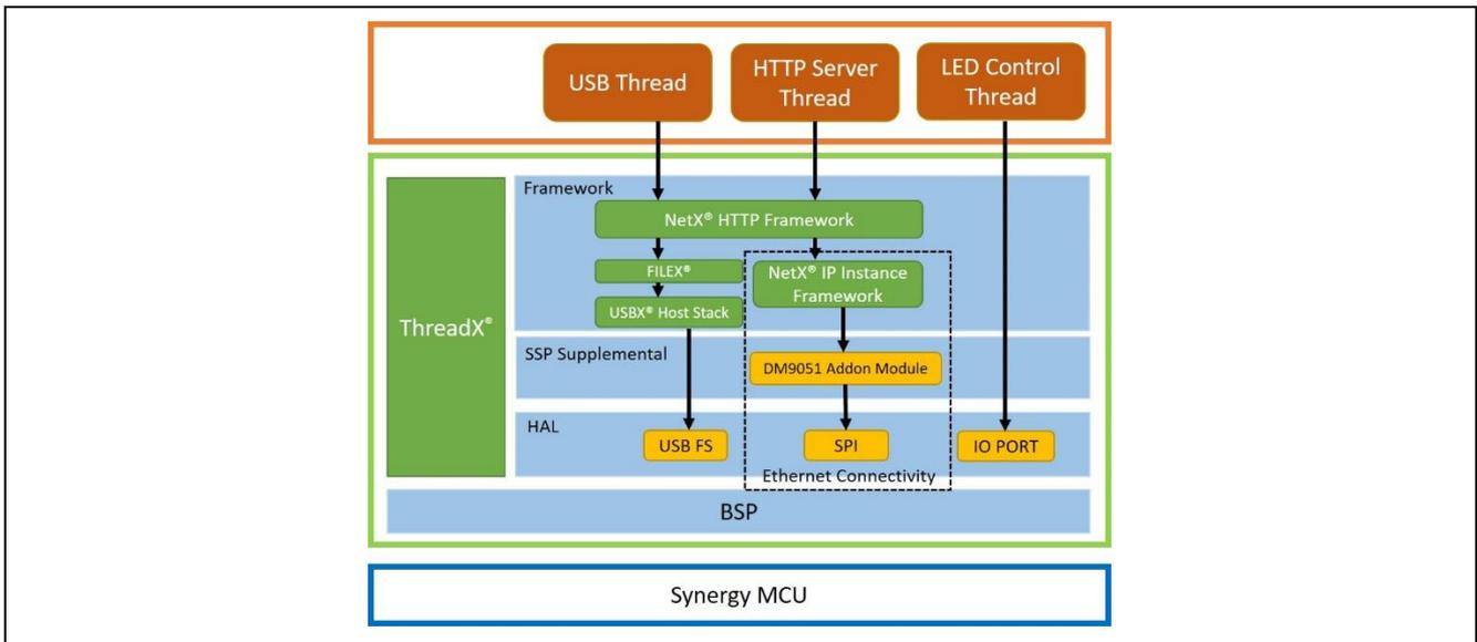
**Figure 5.1 Architecture of NetX Webserver application on DK-S3A7**
