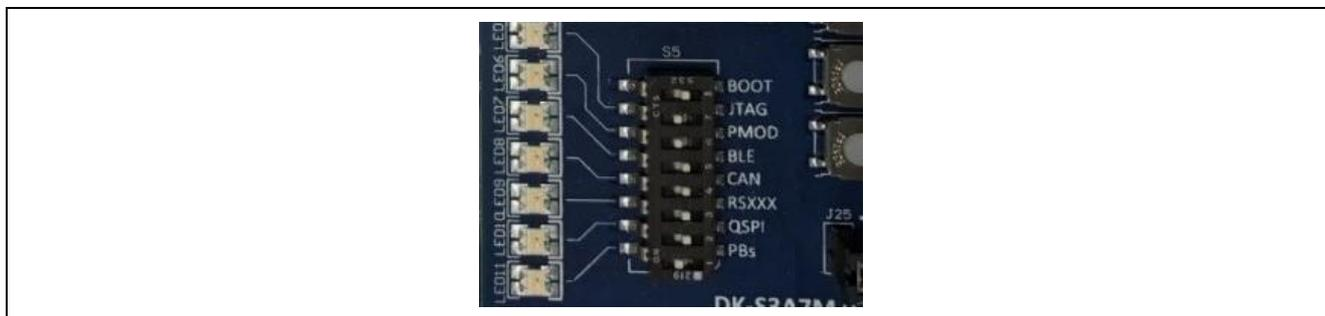
**Figure 4.4 The setting of DIPSW S5 for the DK-S3A7**
