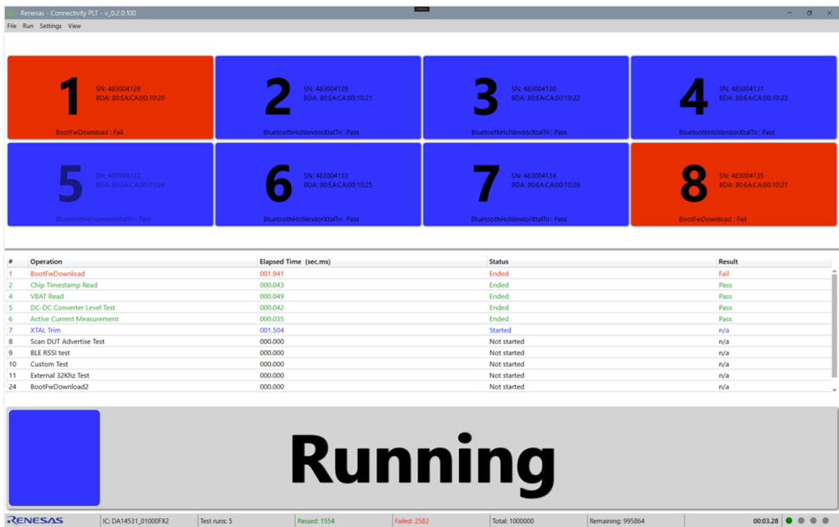
Figure 92. DUTs fail during execution
