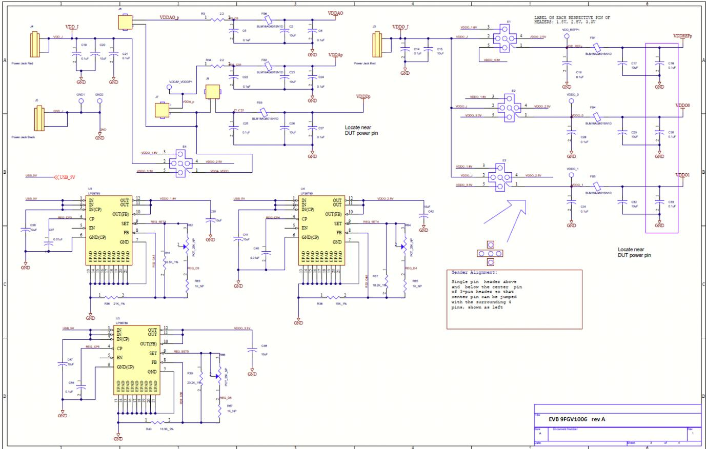
Figure 7. 9FGV1006 PCIe Evaluation Board Schematic – page 4
