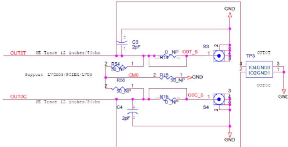
The circuit is designed for maximum flexibility when testing all possible logic types. Default assembly uses a 0.1 $\mu$ F capacitor in place of R14 and R16, and the short across R14 and R16 is cut. No other devices are assembled. This simple AC-coupled configuration allows for testing phase noise and jitter of all possible logic types. The circuit can be modified for custom tests. TP3 is a position to place a differential FET probe.
