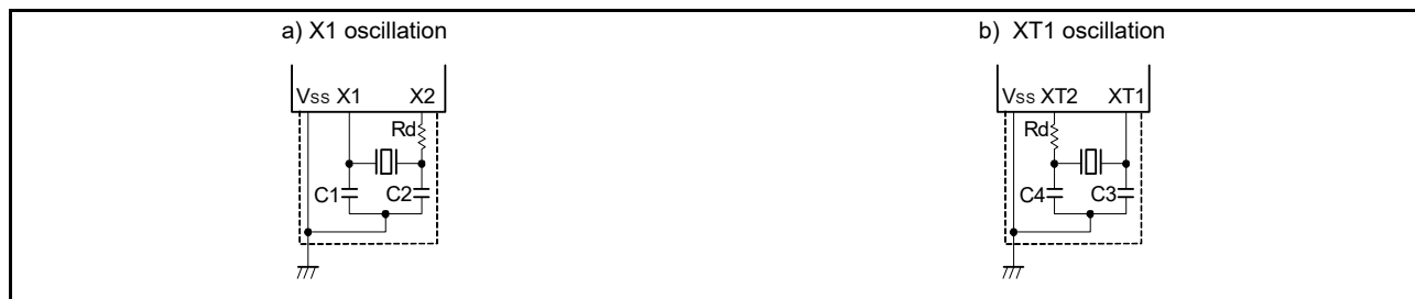
Figure 6 - 23 Examples of External Circuits
