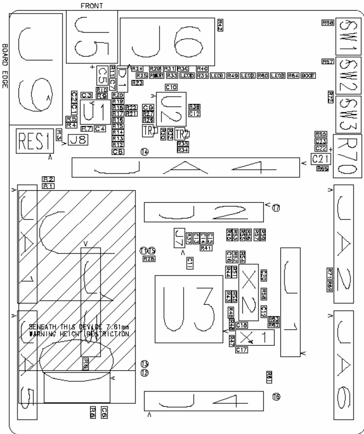
Figure 11-1: Component Placement
