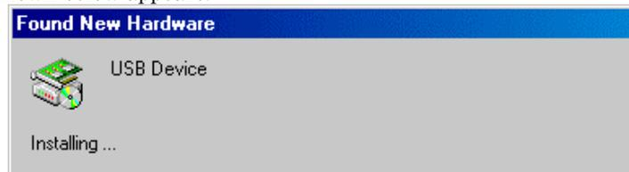
Go on following the wizard, and a dialog box for specifying the setup information file (inf file) is displayed. Specify the musbdrv.inf file stored in a location below the directory where the PDxx is installed (e.g., c:\¥mtool¥pdxx¥drivers).
