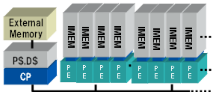
Figure 2 IMAP System Configuration in SIMD Mode
