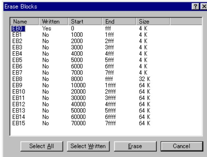
**Note** To erase all blocks, clicking the 'Select All' button inversely displays all blocks. To erase the programmed block, clicking the 'Select Written' button inversely displays the target block.
