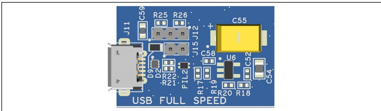
**Figure 16. USB Full Speed Connector**
