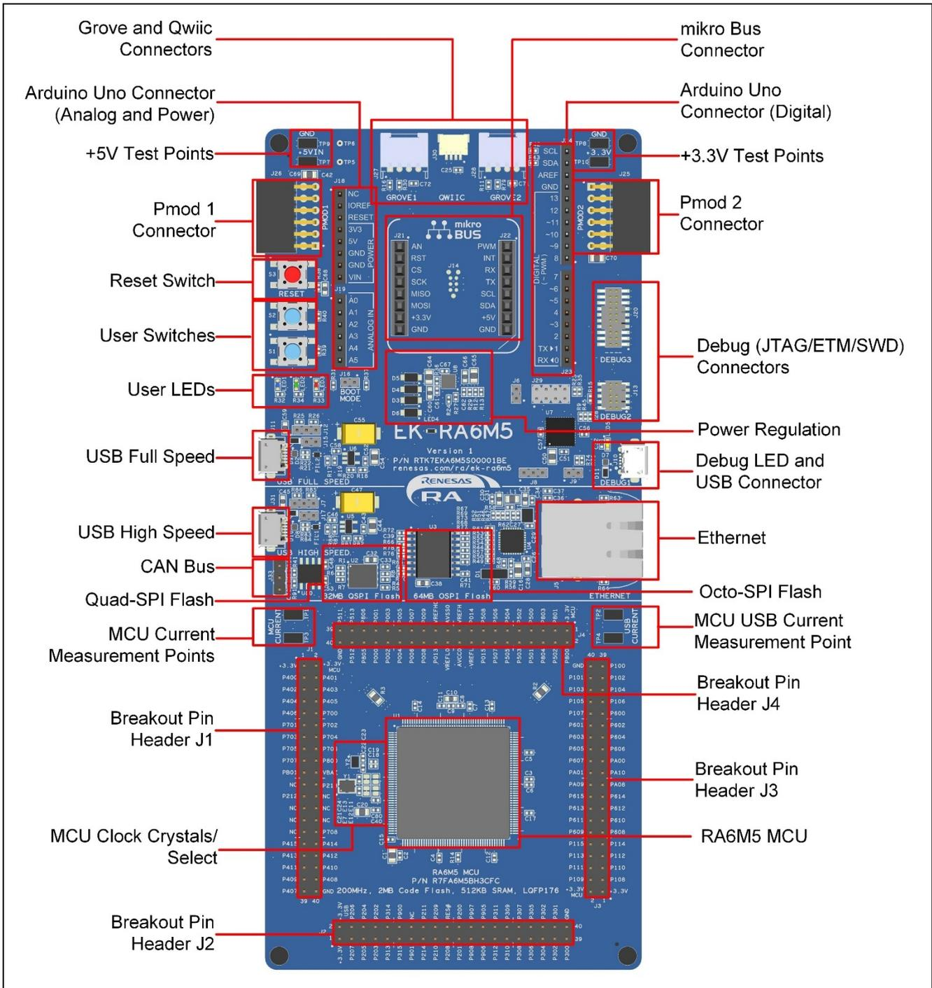
Figure 1. EK-RA6M5 Board Top Side
