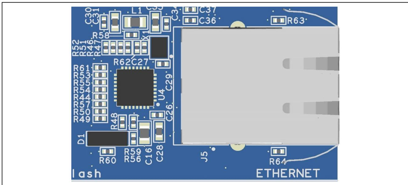
**Figure 22. Ethernet Connector**
