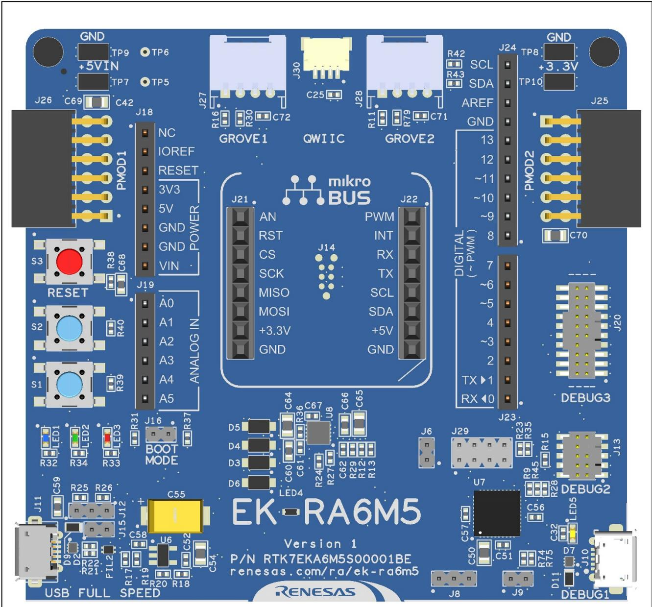
Figure 7. System Control and Ecosystem Access Area
