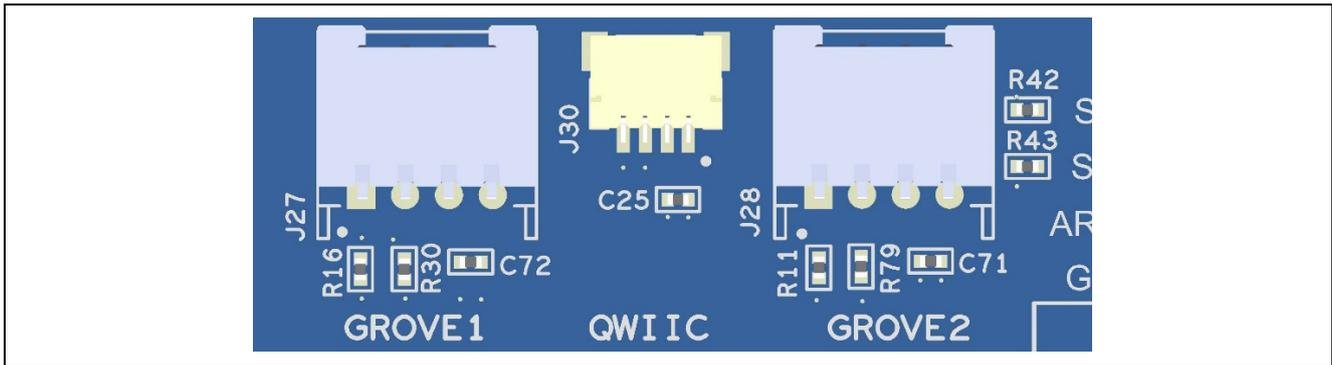
Figure 11. Seed Grove and SparkFun® Qwiic Connectors
