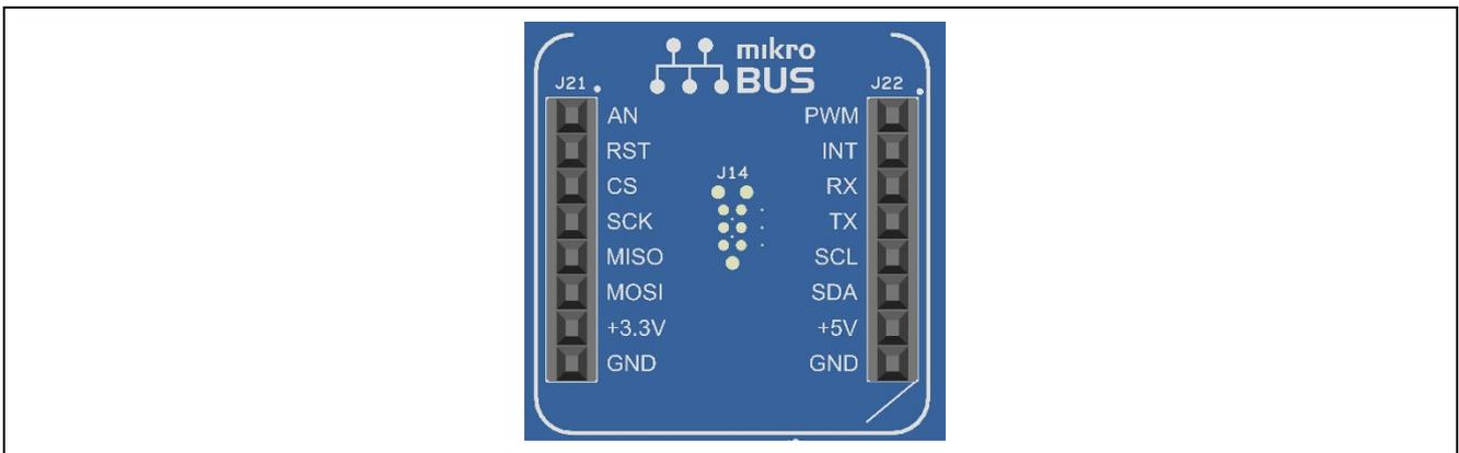
Figure 15. mikroBUS Connection
