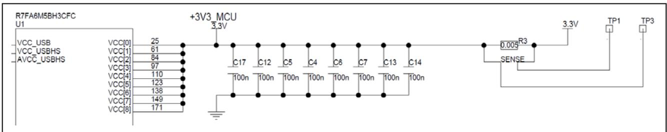
Figure 29. RA +3.3 V Current Measurement Circuit
