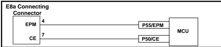
Figure 4.6 Connection of E8a Emulator and Pins P50 and P55 (Single Power Supply and Single-chip Mode)
