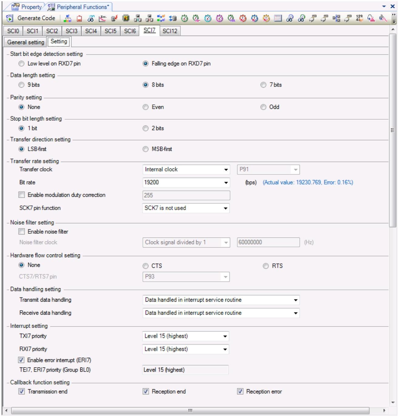
Figure 4-12 SCI7 Asynchronous Setting
