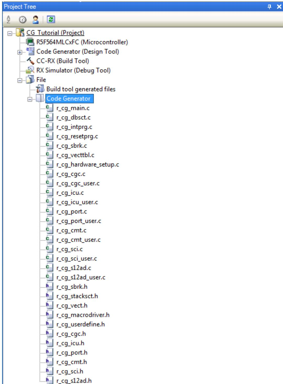
Figure 4-17 Code Generator Files in the Project Tree
