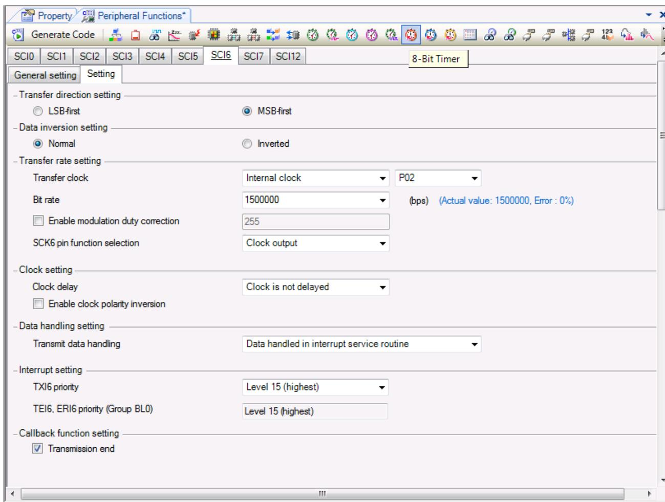
Figure 4-10 SCI6 SPI Master Setting
