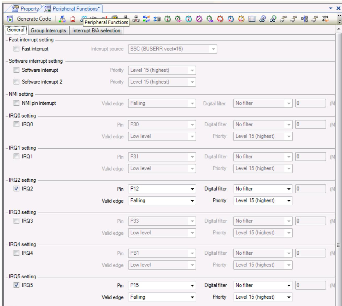
Figure 4-3 Interrupt Functions tab
