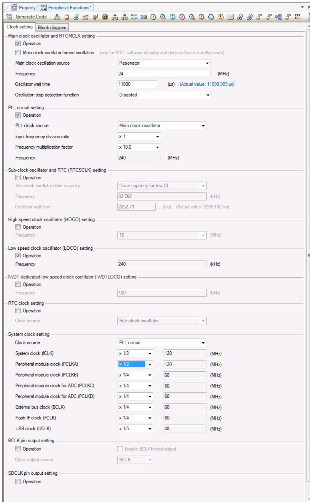
Figure 4-2 Clock setting tab
