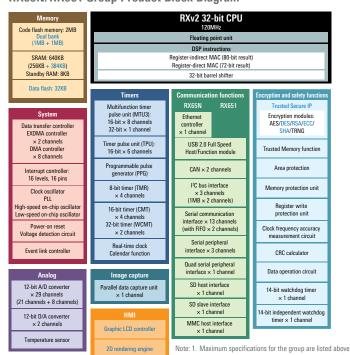
Items printed in blue are not implemented on code flash memory is less than 1.0MB products.
