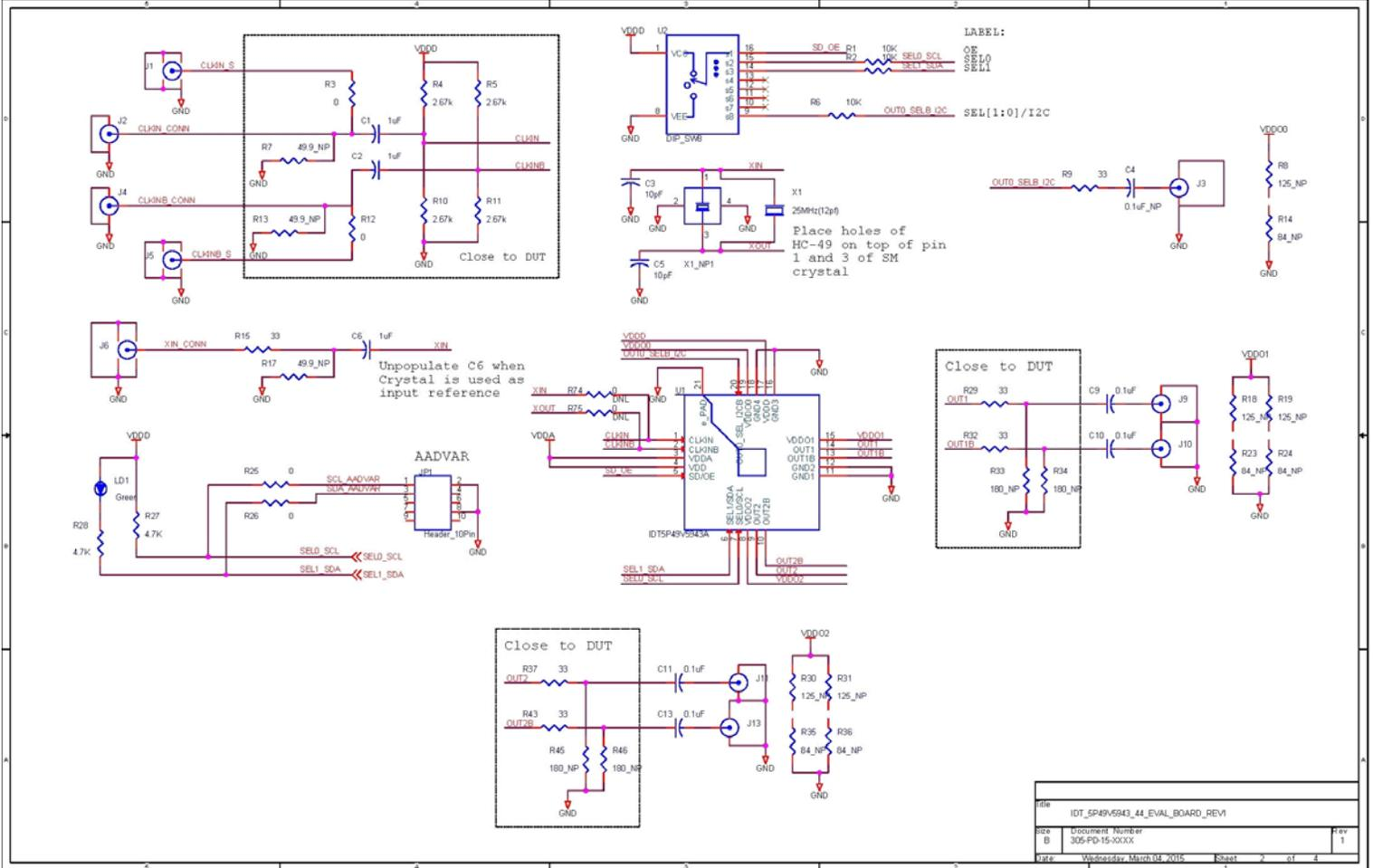
Figure 6. 5P49V5943/44 VersaClock 5 Evaluation Board Schematics – Page 2
