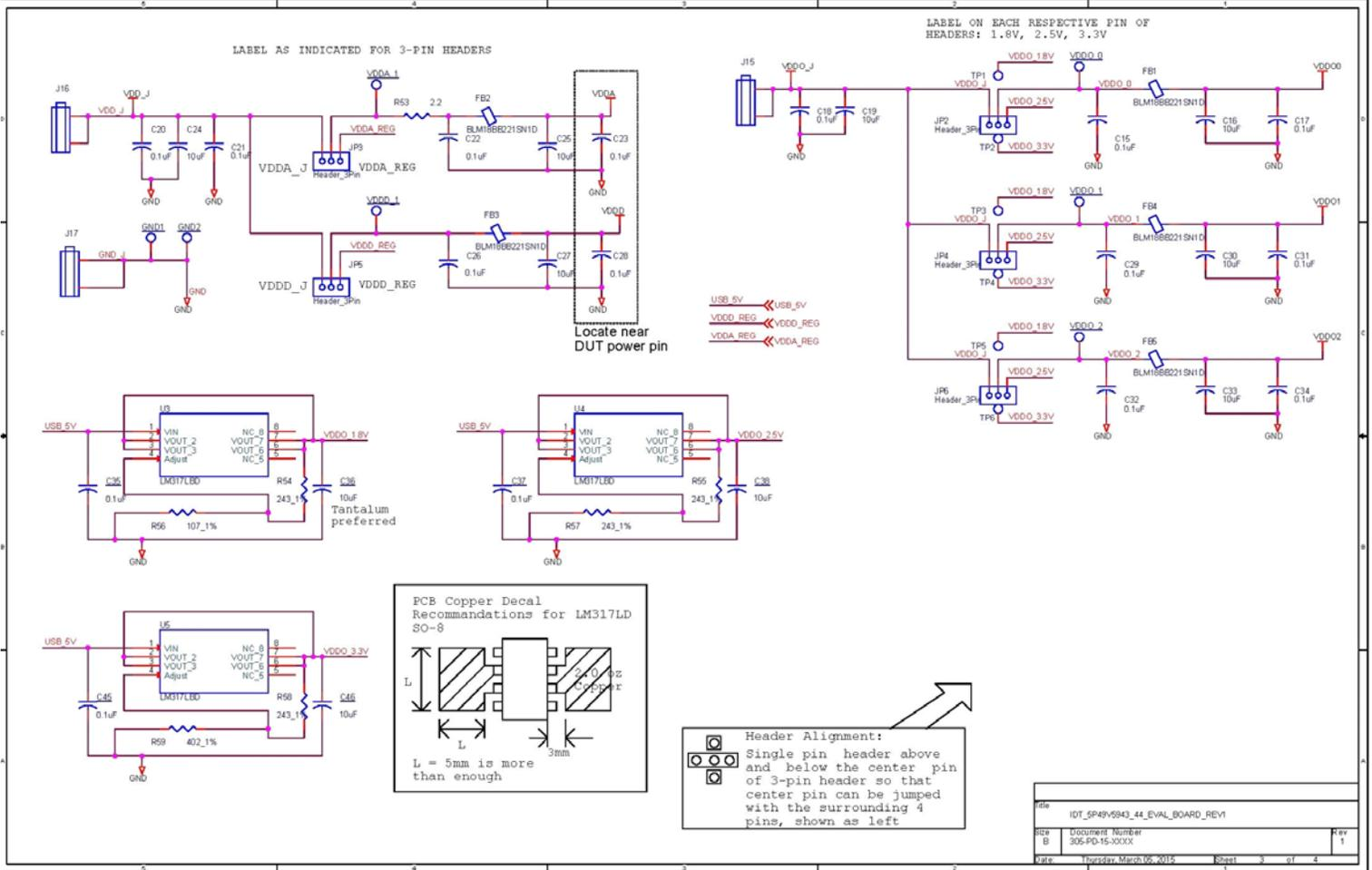
Figure 7. 5P49V5943/44 Evaluation Board Schematics – Page 3
