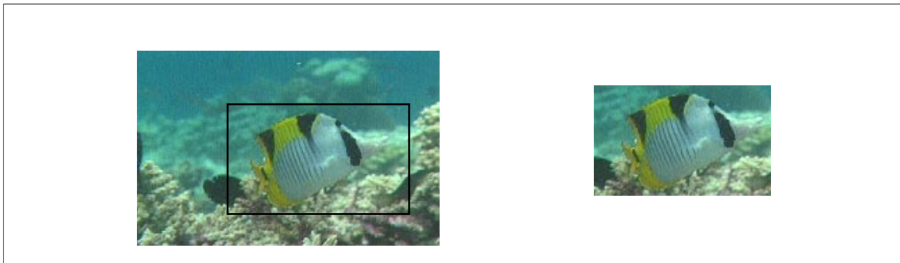
Figure 2-36. Example of Expansion in Expansion Mode 5
