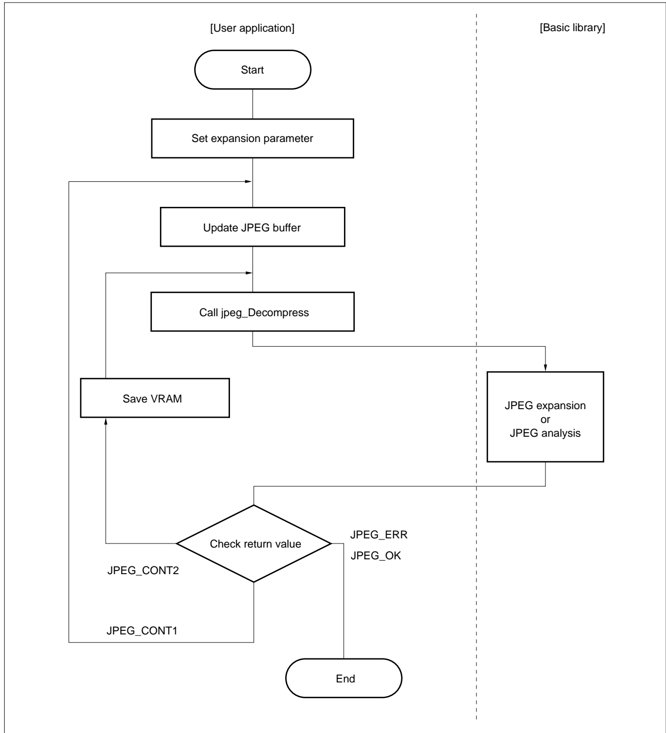
Figure 2-29. Basic Expansion Processing Flow
