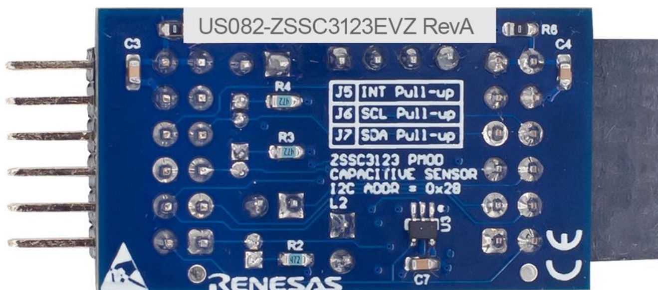
Figure 5. US082-ZSSC3123EVZ Pmod Board Image (Bottom)
