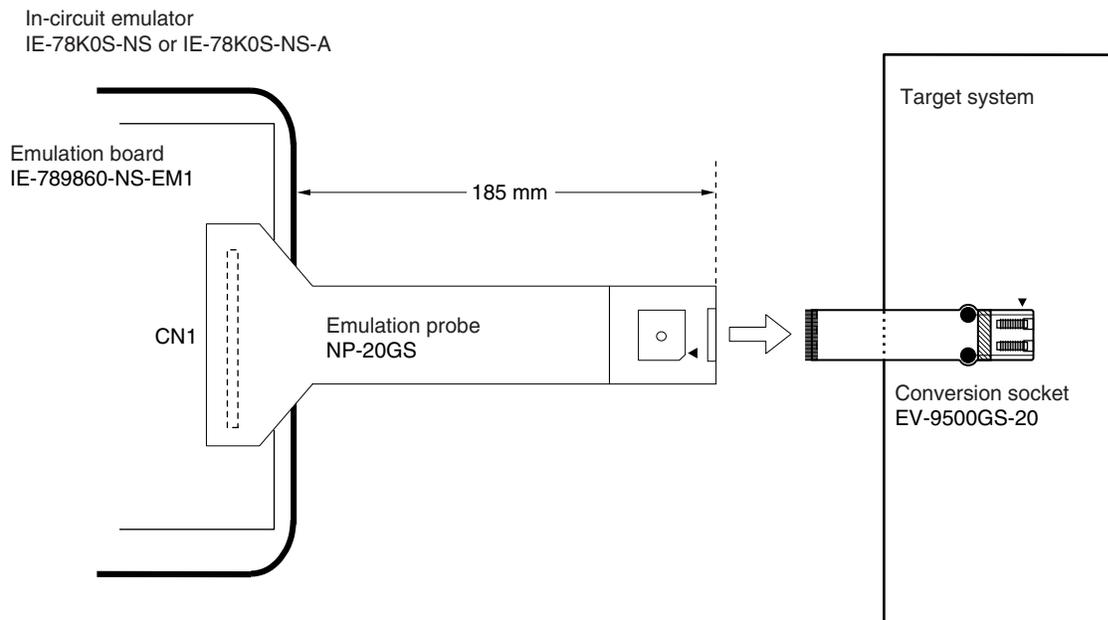
Figure B-2. Connection Conditions of Target System
