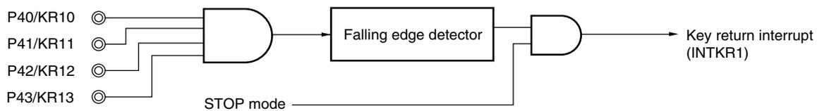
Figure 13-2. Generation Timing of Key Return Interrupt
