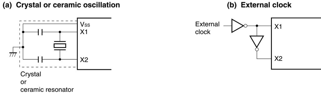
**Caution** When using the system clock oscillator, wire as follows in the area enclosed by the broken lines in Figure 7-3 to avoid an adverse effect from wiring capacitance.
