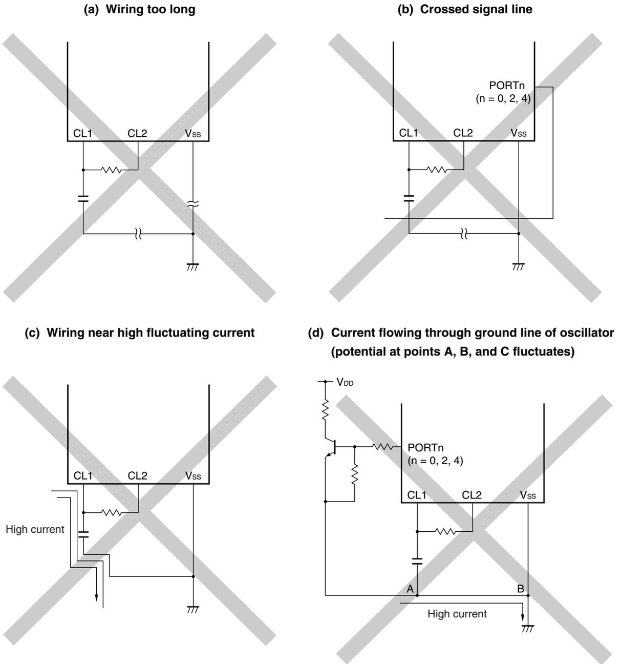
Figure 8-4. Example of Incorrect Resonator Connection (2/2)
