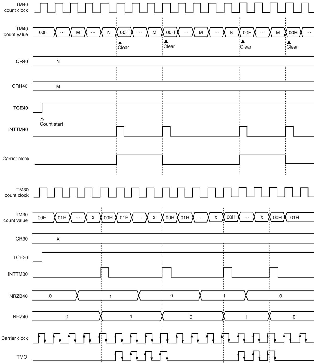
**Remark** This timing chart shows an example in which the value of NRZ40 is changed while the carrier clock is high.
