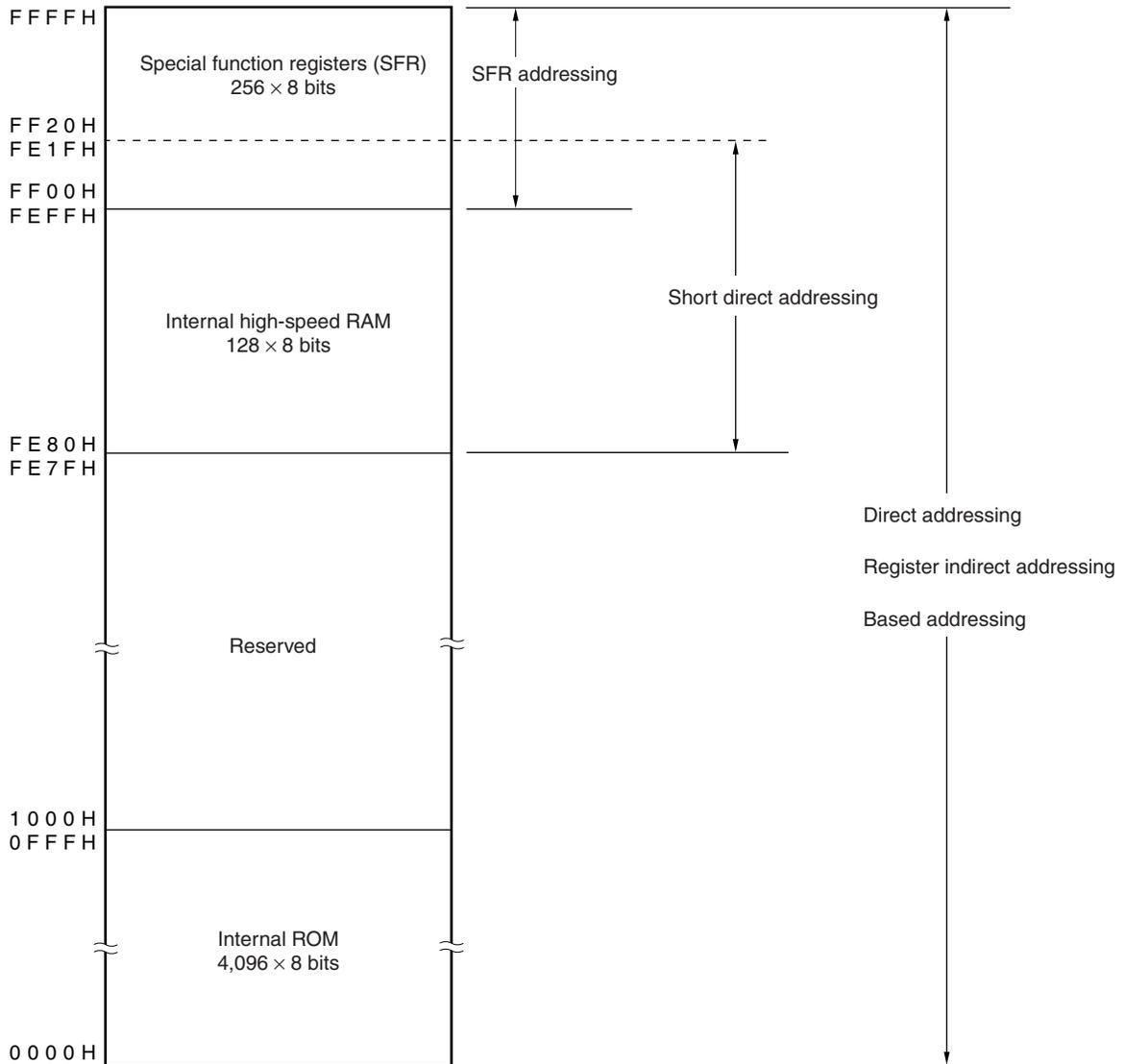
Figure 4-4. Data Memory Addressing ( $\mu$ PD78E9860A, 78E9861A)
