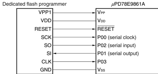
**Note** When supplying the system clock from a dedicated flash writer, connect the CLK and X1 pins and cut off the resonator on the board. When using the clock oscillated by the on-board resonator, do not connect the CLK pin.
