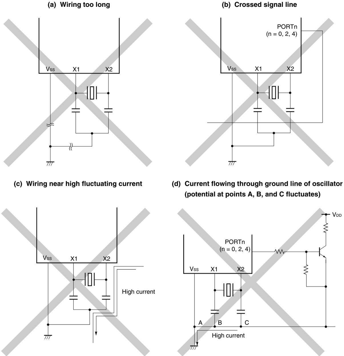
Figure 7-4. Example of Incorrect Resonator Connection (2/2)
