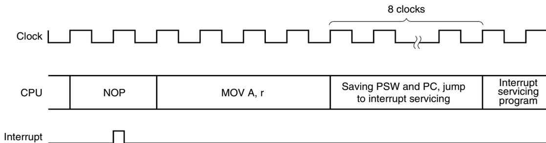
If an interrupt request flag ( $\times\times IF$ ) is set at the last clock of the instruction, the interrupt acknowledgement processing starts after the next instruction is executed.
