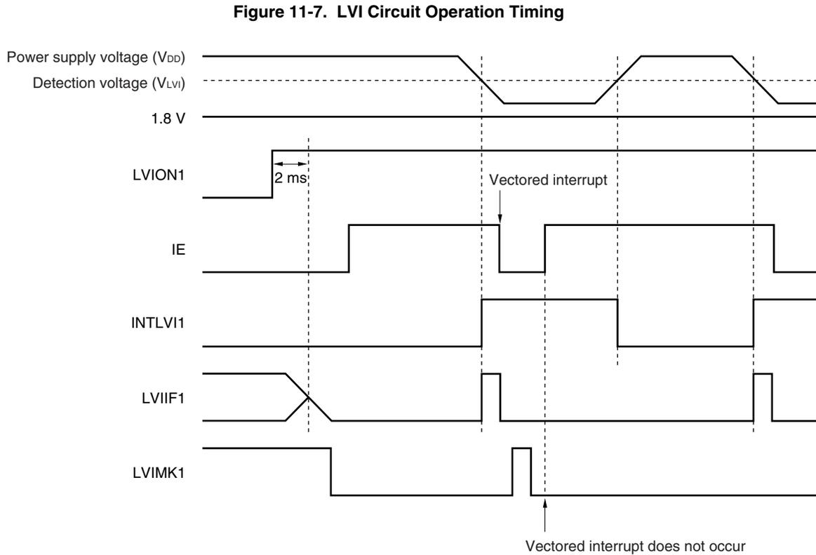
**Caution** The low-voltage detection interrupt request flag (LVIIIF1) is set at the rising edge of the LVI circuit comparator output signal (INTLVI1). Therefore, the power supply voltage ( $V_{DD}$ ) becomes lower than the detection voltage ( $V_{LVI}$ ) during LVI operation, and if that state continues after INTLVI1 generation, LVIIIF1 is not set. After low-voltage detection, when set as  $V_{DD} > V_{LVI}$  and then  $V_{DD} < V_{LVI}$  again, LVIIIF1 is set.
