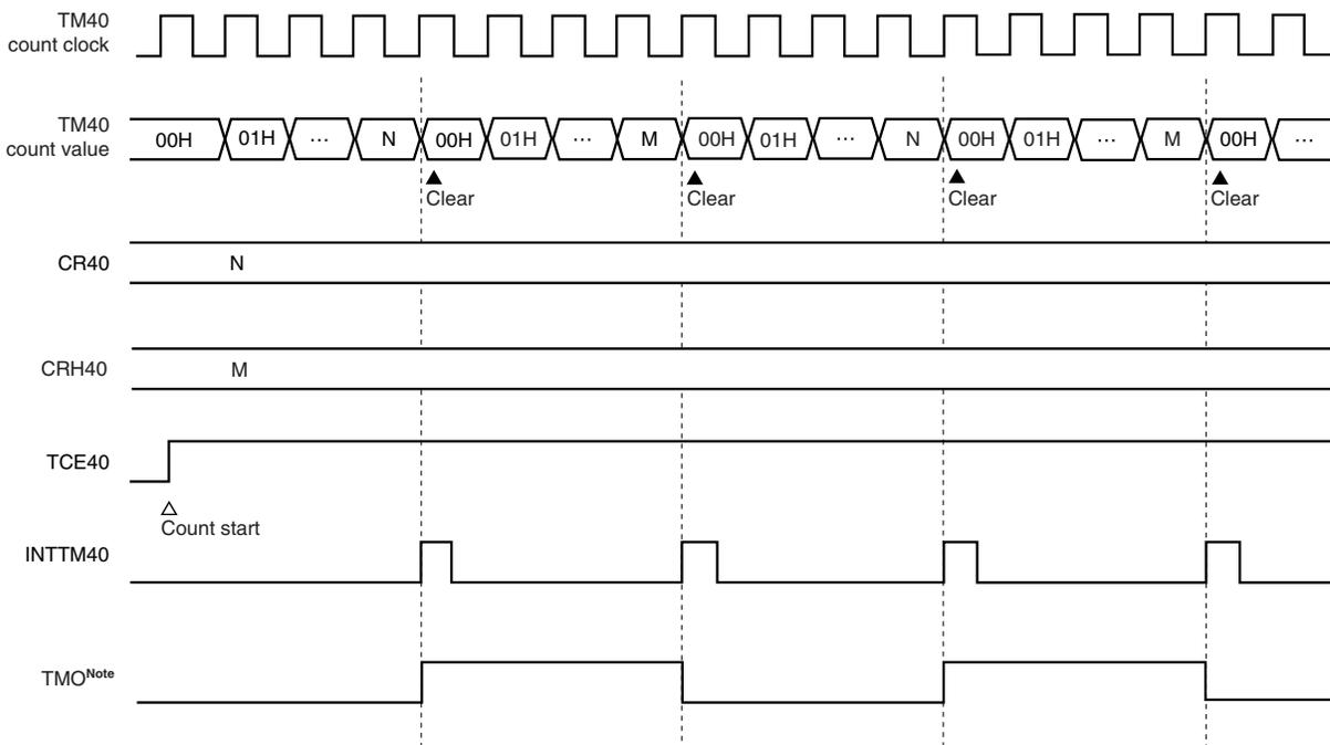
**Note** The initial value of TMO is low level when output is enabled (TOE40 = 1).
