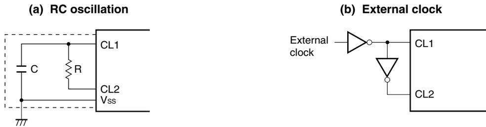
**Caution** When using the system clock oscillator, wire as follows in the area enclosed by the broken lines in Figure 8-3 to avoid an adverse effect from wiring capacitance.
