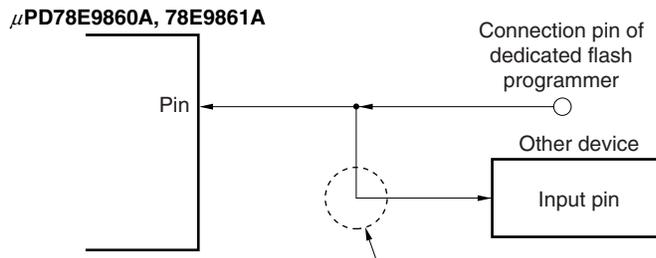
If the signal output by the dedicated flash programmer affects another device in the EEPROM programming mode, isolate the signals of the other device.
