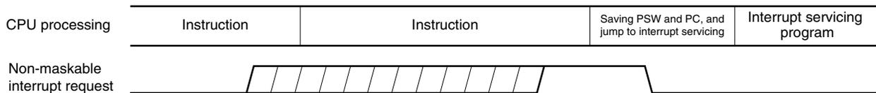
Figure 14-7. Acknowledgement of Non-Maskable Interrupt Request
