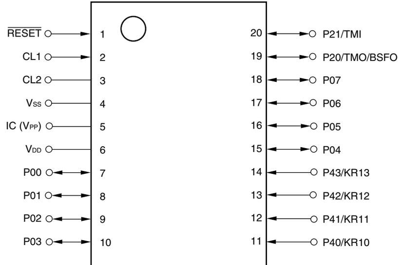
**Caution** Connect the IC (Internally Connected) pin directly to Vss.
