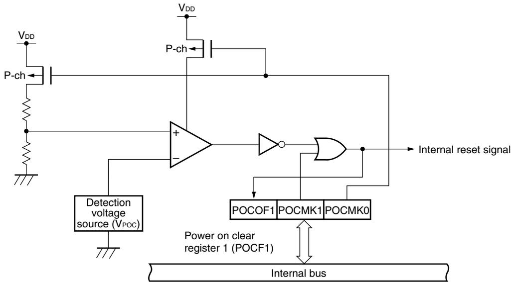
Figure 11-2. Block Diagram of Low-Voltage Detection Circuit
