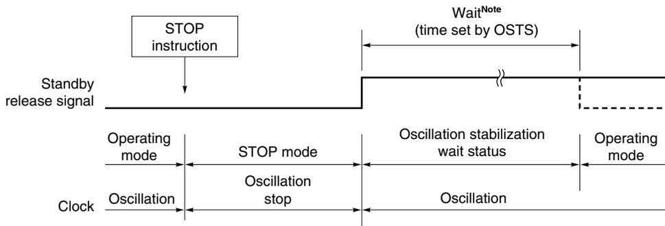
**Note** There is no OSTs in the  $\mu$ PD789062 Subseries, and the wait is fixed at  $2^7/f_{cc}$ .
