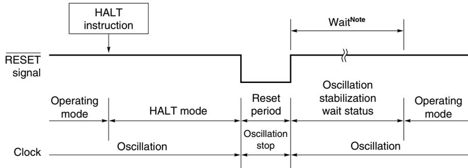
**Note** In the  $\mu\text{PD789052}$  and  $78\text{E9860A}$ ,  $2^{15}/f_x$ : 6.55 ms (@  $f_x = 5.0$  MHz operation)
