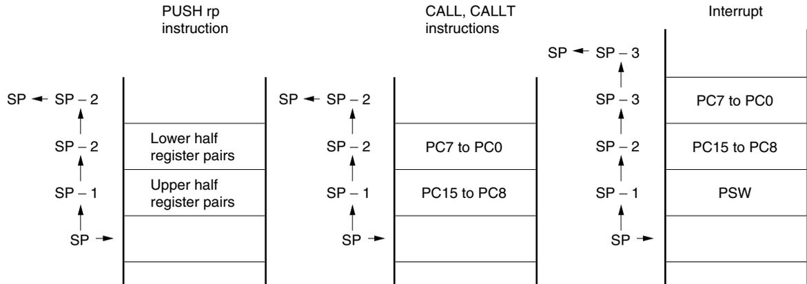
**Figure 4-9. Data to Be Restored from Stack Memory**
