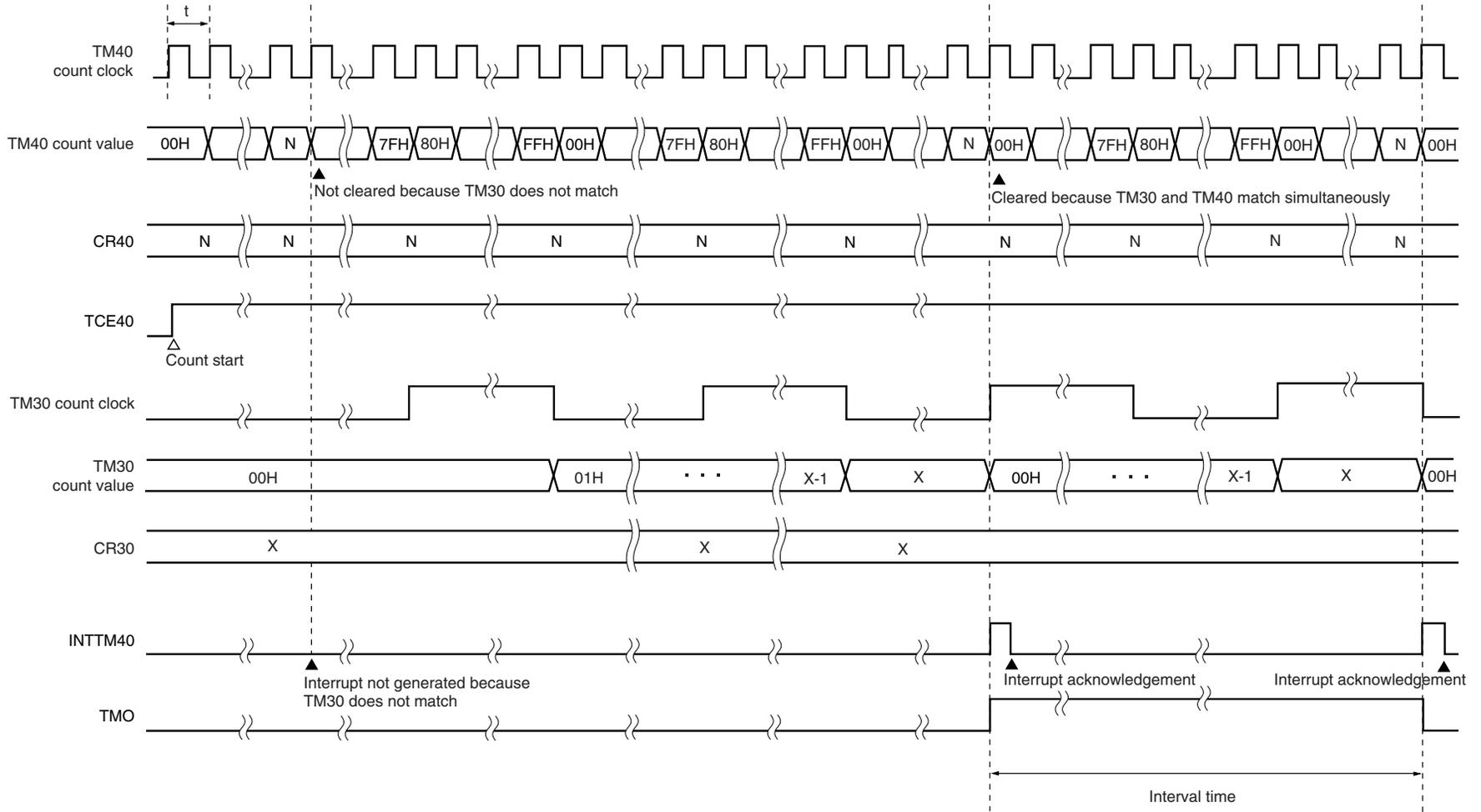
**Remark** Interval time:  $(256X + N + 1) \times t$ : X = 00H to FFH, N = 00H to FFH
