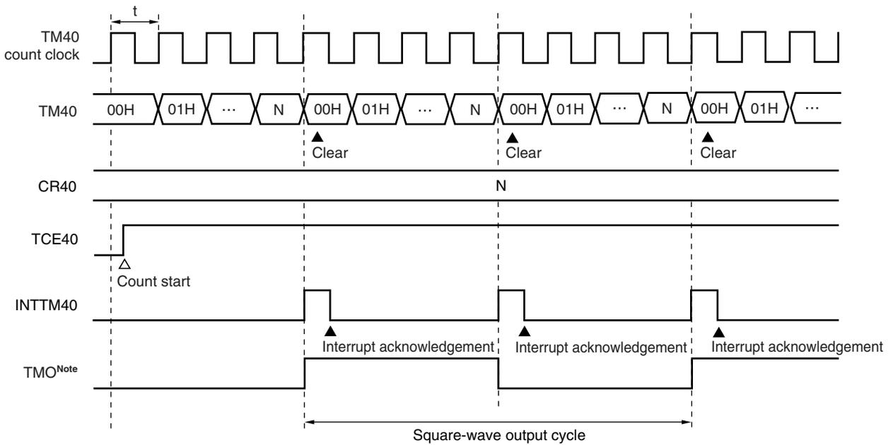
**Note** The initial value of TMO is low level when output is enabled (TOE40 = 1).
