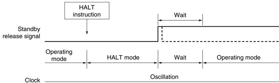
**Remarks** 1. The broken lines indicate the case where the interrupt request that has released standby mode is acknowledged.
