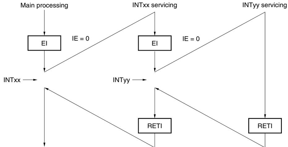
During interrupt  $INT_{xx}$  servicing, interrupt request  $INT_{yy}$  is acknowledged, and multiple interrupts are generated. The EI instruction is issued before each interrupt request acknowledgement, and the interrupt request acknowledgement enable state is set.
