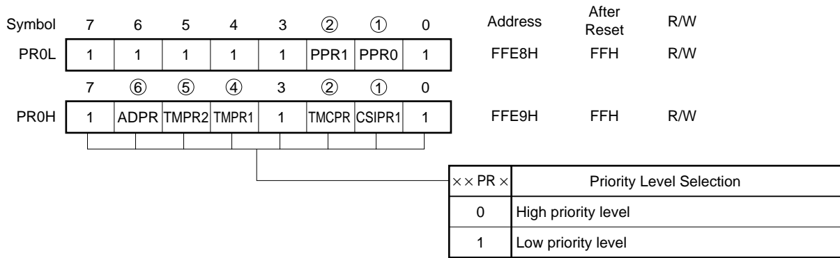
Figure 11-4. Priority Specification Flag Register (PR0L, PR0H) Format
