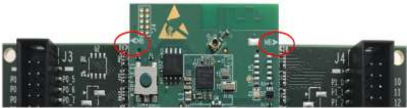
Figure 3: Main board - daughter board alignment
