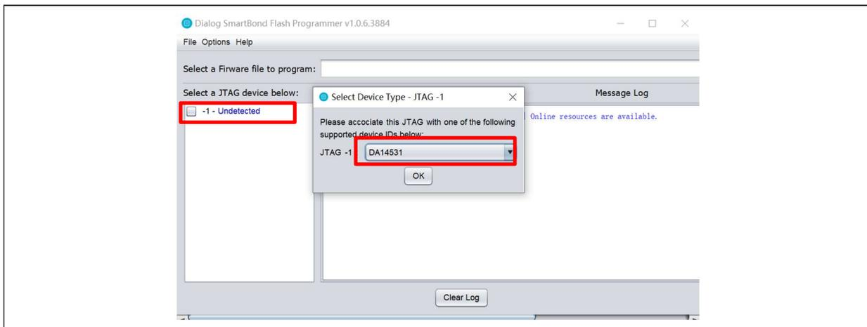
Step 3. Check the selected JTAG device, and then select the “CN051-3 Smart Rangefinder Solution\_v1.0.bin” file by Browse.
