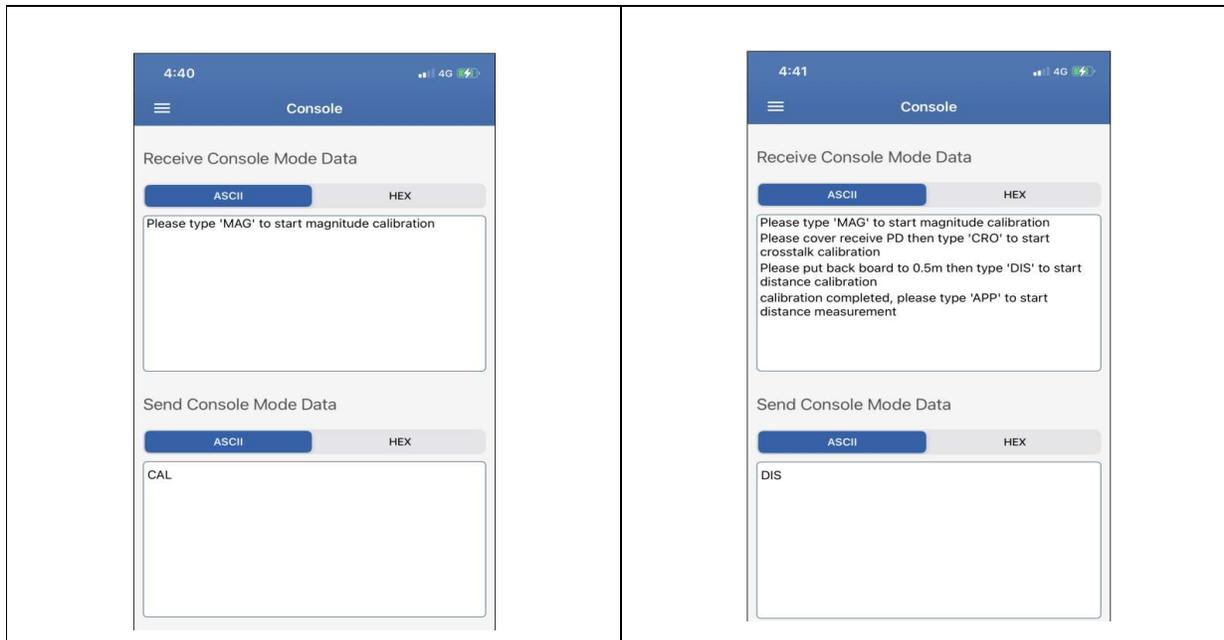
Step5. After distance calibration completed, “calibration completed, please type ‘APP’ to start distance measurement” will show in receive window. After “APP” typed, measurement data display just as bellow.
