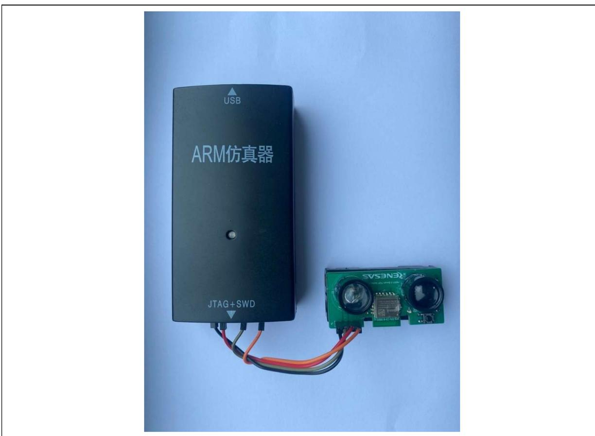
Step 2. Open Dialog SmartBond Flash Programmer, if JTAG device is undetected automatically, click it and select DA14531.
