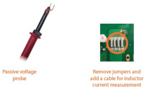
Figure 12. VGS and VDS of Low Side GaN FET Measurement Socket Tips and PFC Inductor Current Measuring Position
