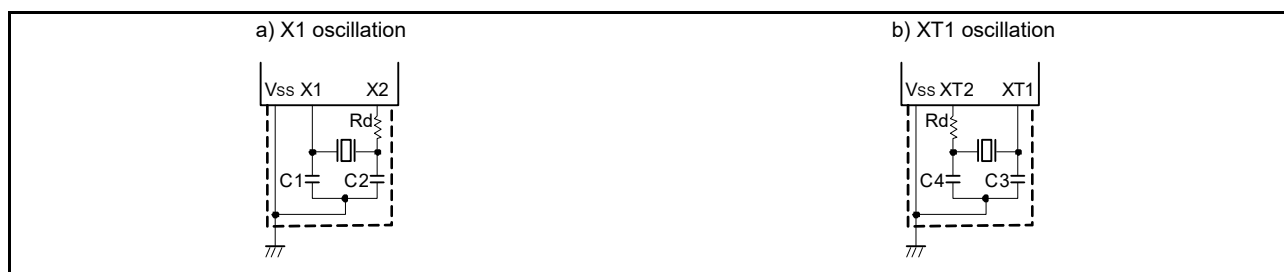
Figure 6 - 26 Examples of External Circuits
