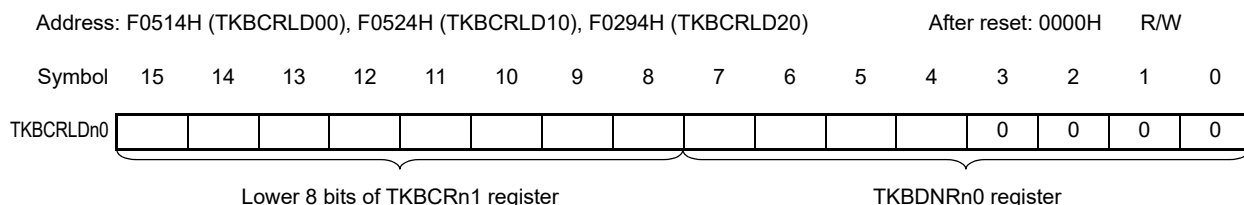
Figure 7 - 18 Format of 16-bit timer KB2 compare 1L & dithering count register n0 (TKBCRLDn0)
