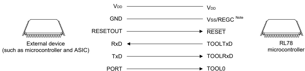
Figure 30 - 4 Communication with External Device
