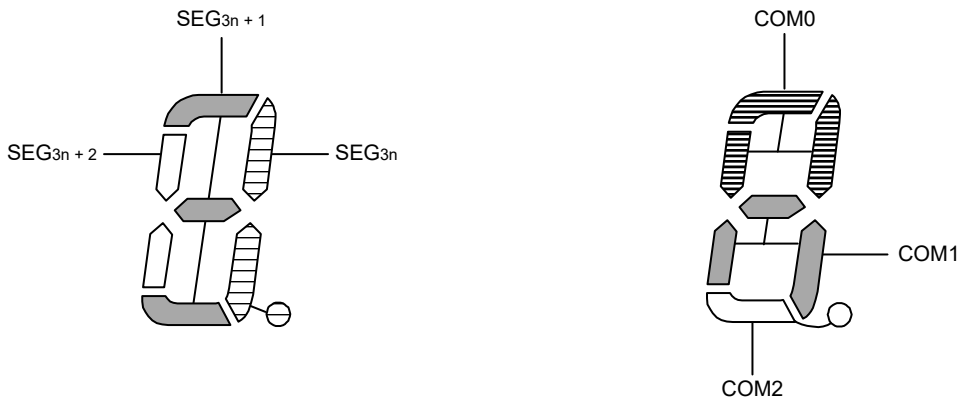
Figure 18 - 36 Three-Time-Slice LCD Display Pattern and Electrode Connections
