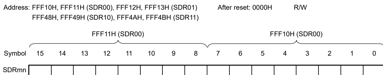
Figure 15 - 11 Format of Serial data register mn (SDRmn)
