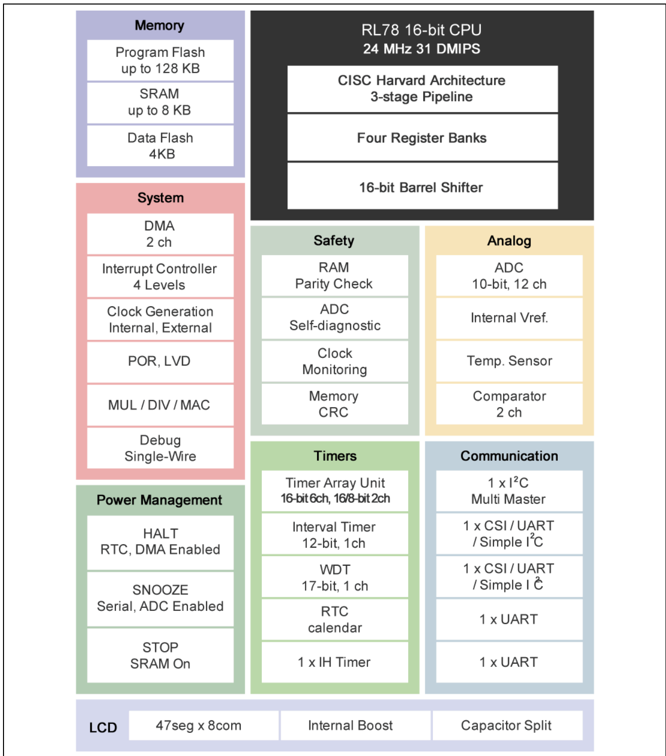
Figure 2.1 RL78/L13 (80-pin products) Block Diagram
