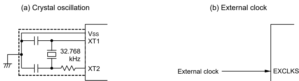
Figure 6-21. Example of External Circuit of XT1 Oscillator
