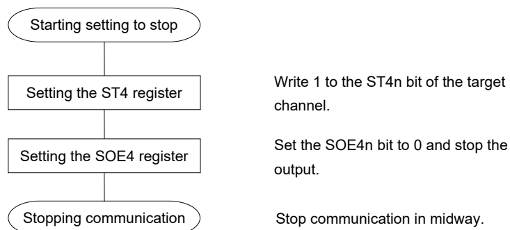
Figure 16-53. Procedure for Stopping DALI Transmission
