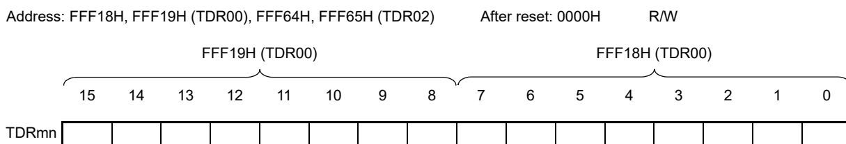
Figure 6 - 8 Format of Timer data register mn (TDRmn) (n = 1, 3)
