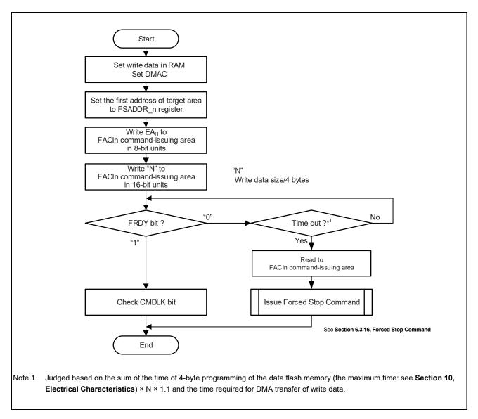
Figure 6.10 DMA Programming Command Usage
