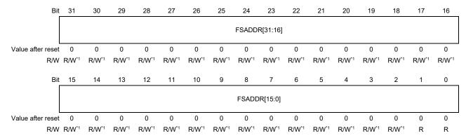
Note 1. Writing to this bit in periods from the first write access of FACI command to FRDY bit in FSTATR\_n register returns to "1" from "0" is ignored. (Except for FRDY = "1" in "Command Lock" state)
