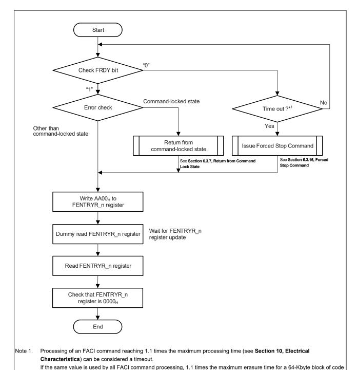
Figure 6.5 Flow of Shift to Read Mode
