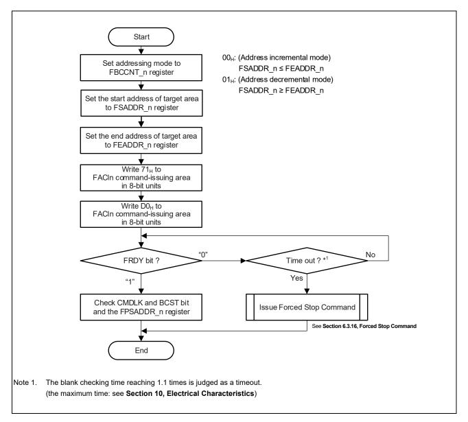
Figure 6.20 Blank Checking Command Usage
