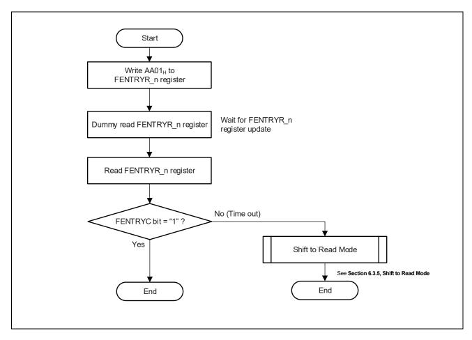
Figure 6.3 Flow of Shift to Code Flash Programming/Erasure Mode
