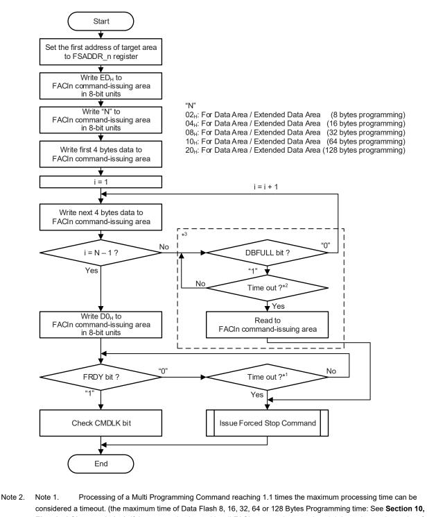
Electrical Characteristics). If the same value is used by all FACI command processing, 1.1 times the maximum time for a 128-byte programming of data flash memory can be considered a timeout.
