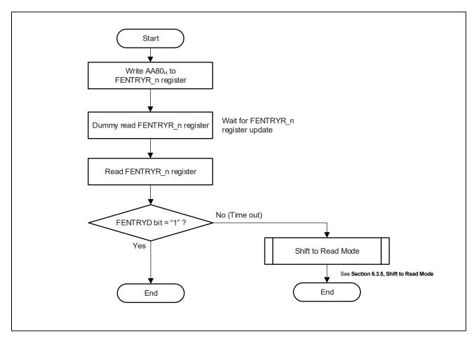
Figure 6.4 Flow of Shift to Data Flash Programming/Erasure Mode
