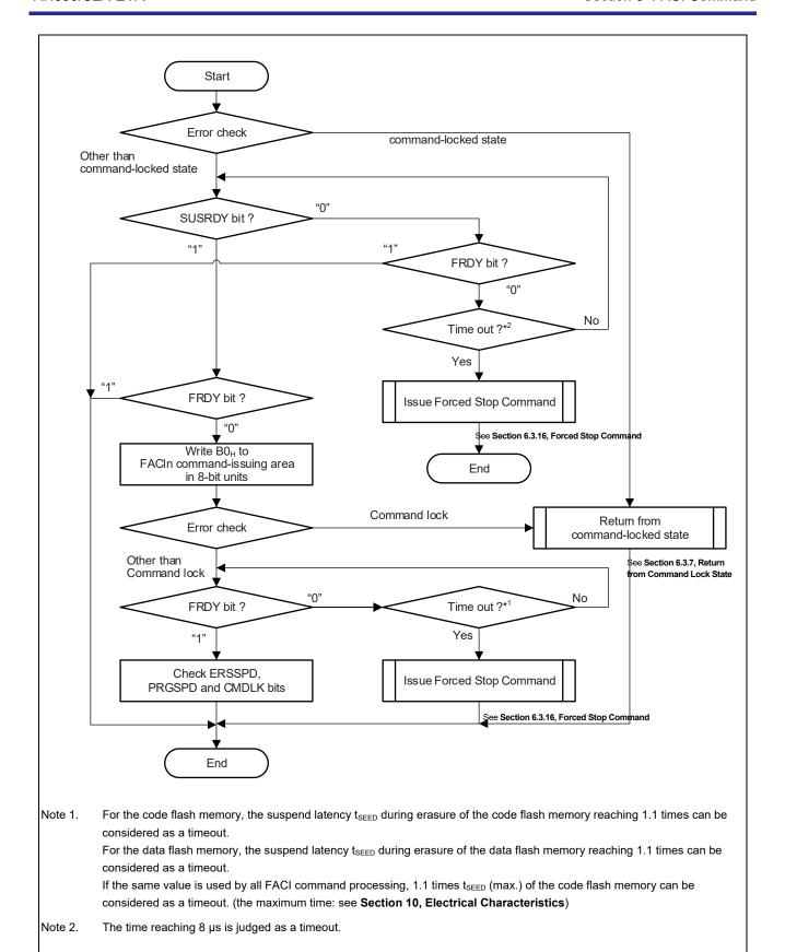
Figure 6.13 Programming/Erasure Suspension Command Usage
