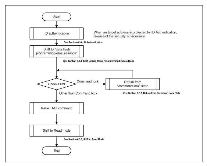
Figure 6.2 Overview of Command Usage in Data Flash Programming/Erasure Mode
