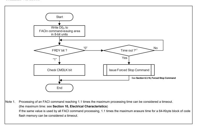
Figure 6.17 Programming/Erasure Resumption Command Usage
