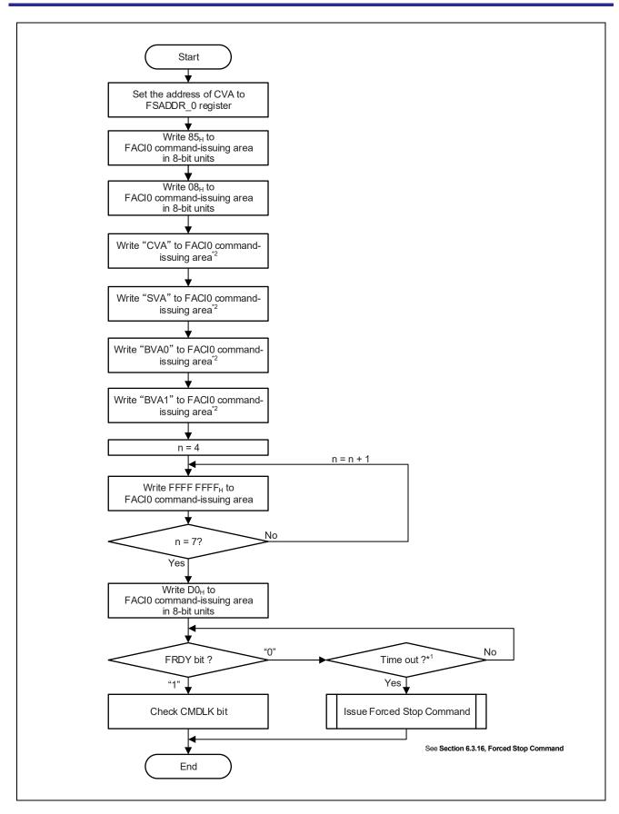
Figure 6.26 Switch Programming Command Usage (1/2)
