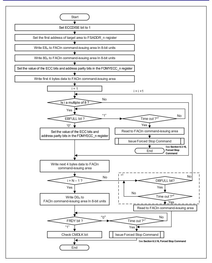
Figure 6.34 Injecting an ECC Error for the Code Flash Memory (1/2)
