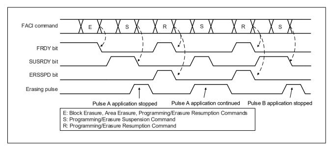
Figure 6.15 Suspend Erasure Command (Suspension-Priority Mode)
