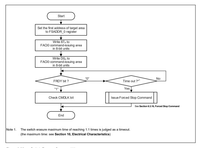
Figure 6.25 Switch Erasure Command Usage
