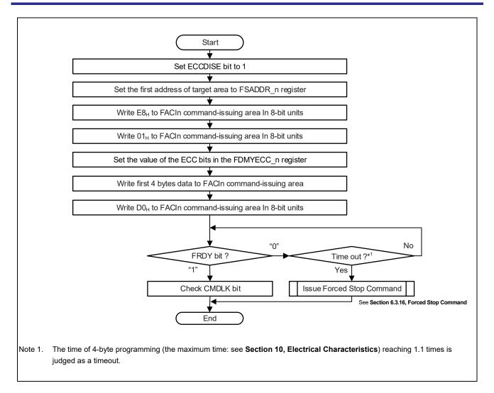
Figure 6.35 Injecting an ECC Error for the Data Flash Memory
